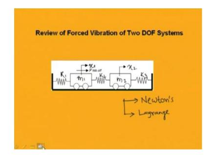
A spring mass system is shown here. So, m 1 and m 2 are the mass of this system. And k 1, k 2, k 3 are the stiffness of the system. Let this mass m 1 is subjected to a harmonic force of F sin omega t. So, in this case already you know to derive this equation motion either you can go for this Newtons method by using the Newtons second law; you can derive the equation motion or you may use the Lagrange principle or the Hamilton extended, Hamilton principle to derive this equation motion.
