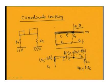
So, if I will take 1 1 equal to 0 that means point C point coincide with the left hand. Then, the equation motion will become so you can see that 1 1 if I will take at 0. So, in that case this equation will becomes like this.
