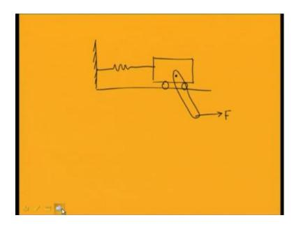
Also we have studied about the normal mode of vibration of a system. And already I have found the equation motion for the systems, I have taken a system this simple spring mass system in which another rod is hanging. And I have found the equation motion using Hamilton principle; also you may use the Lagrange principle to find this equation motion.
