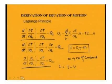
So, previously I told you about the Lagrange principle; using Lagrange principle you can find the equation motion either you can use this from this kinetic energy. And this generalized force you can find the equation motion or you can use the Lagrangian on the system which is equal to L equal to T minus V; T is the kinetic energy, V is the potential energy. So, you can use this expression to find the equation motion.
