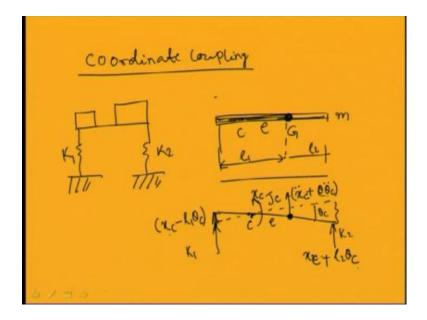
And, taking the moment above this point c; I can take the moment about this point c. So, moment about this point will be equal to 0. So, moment of all the forces about this point I can take so this will be equal to J c into theta c double theta c double dot plus this mass
