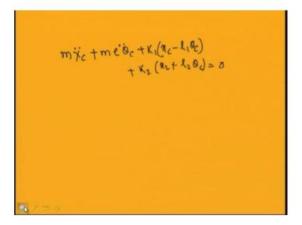
So, by doing the force balance I can write m into X c double dot plus m e theta c double dot plus k 1 into x c minus l 1 theta c plus k 2 into x 2 plus l 2 theta c equal to 0.
