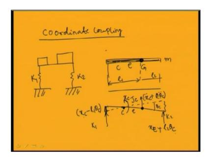
So, in this case you just observe that by taking a coordinate system at position C. So, I am taking a coordinate point at or I am describing the motion of the system by taking a coordinate system here; that is the displacement translational displacement x c and rotational displacement theta c.
