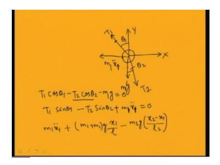
In case of normal mode vibration both the masses; this m 1 and m 2 will move with same frequency and will pass the equilibrium position at the same time. So, this is this is the normal mode we are assuming, and the actual vibration or actual free vibration will depend on the initial conditions that thing already we have seen.
