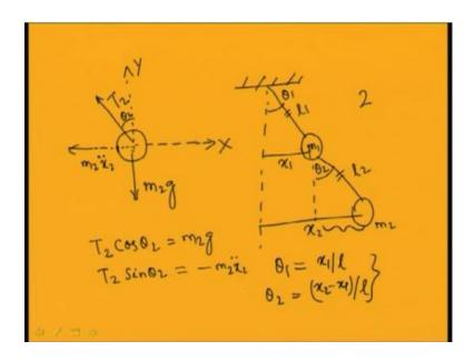
Previous case you have m 2 x 2 double dot. So, for this first for the first mass it is equal to m 1 m 1 x 1 double dot and so this is equal to T 1 cos theta 1 minus T 2 cos theta 2 this is equal to minus m 1 g. So, this is equal to this weight equal to m 1 g. So, this becomes as T 2 equal to m 2 g. So, this becomes T 1 becomes m 1 g plus m 2 g.
