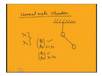
So, using these normal modes last class we have also find; we have also found the free vibration response of a system and normal mode vibration. So, using the normal mode vibration; so for this case we have taken the double pendulum. So, in case of double pendulum we have derived the equation motion using Lagrange principle. And from that we have found the normal modes of the system. So, in case of normal. So, we have found 2 normal mode vibration; so one we got lambda 1 and lambda 2.
