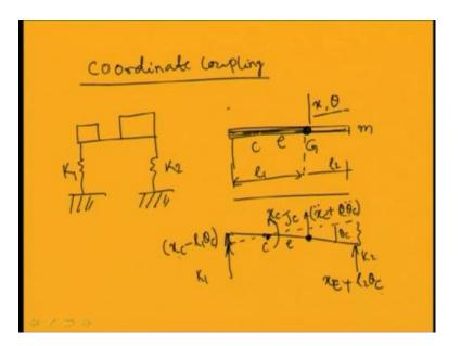
That means, if I take the coordinate system at point G instead of taking at point C. So, if I will take the coordinate position here, and I will describe this motion in terms of x; and theta rotation displacement x here and rotation theta here.
