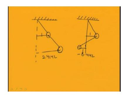
So, if we draw these modes of the first case you can see that; the first case the opposite way also you can do. So, when X 1 becomes 1; so this X 2 will becomes. So, when X 1 equal to 1, X 2 equal to 2; so this X 2 equal to 2.4142 that is 1 by 0.4 1 4 2 equal to 2.4142. And for the second mode you can see that so when this is equal to 1. So, this becomes you can find this; so you can see that this becomes minus0.4142. So, X 2 becomes minus 0.4142.
