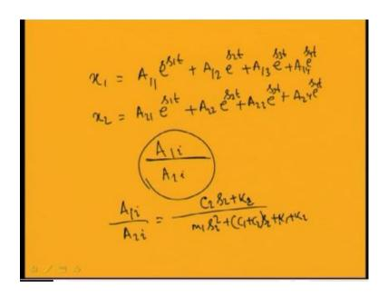
So, from these equation you can write A 1 i by A 2 i is equal to c 2 s i plus k i k 2 by this m 1 s i square plus the C 1 plus C 2 s i plus k 1 plus k 2. So, in this way you can determine the response of a system with damping. So, next class we will study, we will take one example solve this damp system, and also will study about the force vibration of 2 degree of freedom system.
