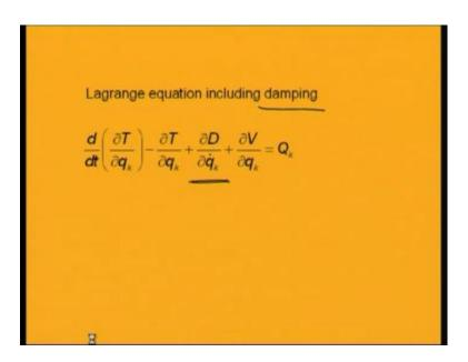
For a system with damping, you can use this dissipation energy to find the equation motion.
