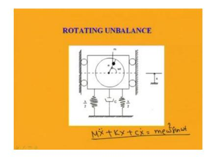
Also we have studied about this rotating unbalance. In case of rotating unbalance in the machine, there is an unbalanced mass placed at a distance e from the center. So, we have
