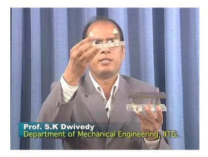
In the single degree of freedom system I have shown the example of a spring mass damper system. So, in this system you can see these are the springs, and this mass is supported on the spring. So, in case of free vibration, I am giving a force and leaving it. So, due to that this mass will vibrate, and in case of forced vibration you are continuously giving a force to the system.
