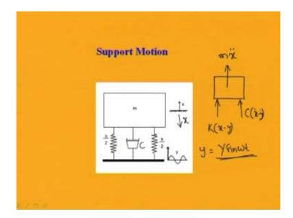
So, let this is the system. So, the system has a mass m. It is supported by the spring with spring constant K and a damper with damping C. So, let the support vibrate with y. So, assume this y equal to Y sin omega t. So, we just assume that the support vibrate in a harmonic way. So, when the support is vibrating in a harmonic manner, then we have to find what is this expression for this X.
