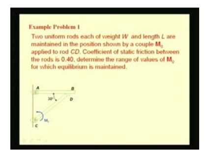
Let us see an example. Here you see two rods AB and CD pinned at A and C. They have a uniform weight of W and they are maintained in a position by the couple  $M_0$  at C. The coefficient of friction occurring between the contacting surfaces is 0.40. We are interested to determine the range of this moment which can maintain this equilibrium.
