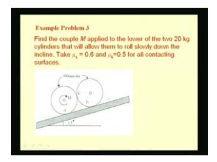
Let us consider another example. Here you see two cylindrical rollers each weighing 20kg kept on an incline whose inclination is 15 degrees. Their diameters are given as 300mm. The values of coefficient for friction, both static and kinetic are given for all the contacting surfaces.
