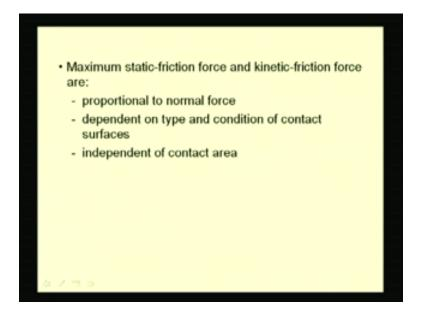
This maximum static-frictional force and the kinetic-frictional force that we have seen are proportional to the normal force, and depend only on the condition of the contacting surfaces, and they are independent of the contact area. This has been found by again series of experiments.
