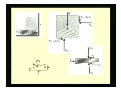
We have this block and the free body diagram of the wedge. Since at both these contact points this wedge C is trying to move from left to right, these frictional forces oppose the same and thus they are marked from right to left. These are the normal reactions. For the impending case this can be related to the normal reaction using this coefficient of friction, mu<sub>s</sub>.
