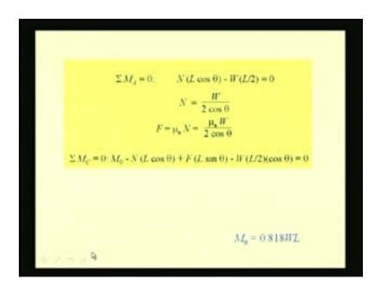
Let us write only those equations which are of interest. We sum the moment about A and equate it to 0. From this we obtain this normal reaction N from the free body diagram 1, which is equal to W by 2 cos theta. We know the relation between the frictional force and the normal force; they are related by this coefficient of static-friction. So the frictional force becomes mu<sub>s</sub> W by 2 cos theta.
