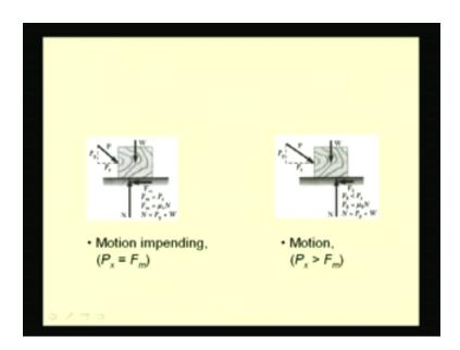
When the motion is impending, at that case we have this  $P_x$  equal to the maximum limiting force  $F_m$ . Only for this impending motion case we have the relation between this frictional force, which is equal to  $F_m$  and N as  $F_m$  equal to  $mu_s$  times of N.
