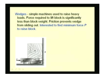
The simplest machines that use friction in order to do some work are wedges. These are devices that are used to raise loads or to keep loads in certain position. They advantageously use friction to accomplish this job. Here in this picture you see this block A which has to be raised or supported in this position. We use these wedges C and D in order to accomplish this task.
