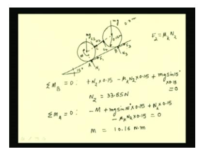
We have the incline, inclined at 15 degrees and the two rollers. At this point of contact for the roller, let us say the normal reaction is  $N_1$  and we have a frictional force  $F_1$  along this incline; because, this cylinder if allowed will try to slip in this direction and the frictional force has to prevent this slippage. At this point of contact, the frictional force is upward along the incline.
