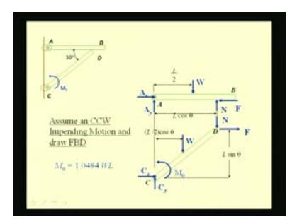
The other impending motion is that this rod CD has a counter clockwise motion. That means this point B tends to move from B to A, thereby the frictional force developed at this contact point is from A to B which is opposite to the impending motion.
