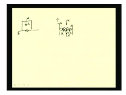
Let us take an object A, which is in contact with another object B. Let us say this is the weight of this object. If we consider microscopically a portion of this contact, there are undulations on the surface of both A and B. The contact actually happens at few of these places and not as seen macroscopically.
