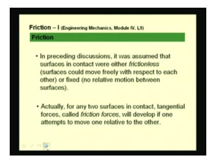
They prevent the relative motion between the two and offer resistance to some degree before a motion impends and starts. This is for all surfaces, irrespective of how smooth they are though the degree of resistance offered for rough surfaces is more and for smooth surfaces, it is less. The origins of these frictional forces are primarily due to the non-uniform nature of the contacting surfaces in the microscopic levels.
