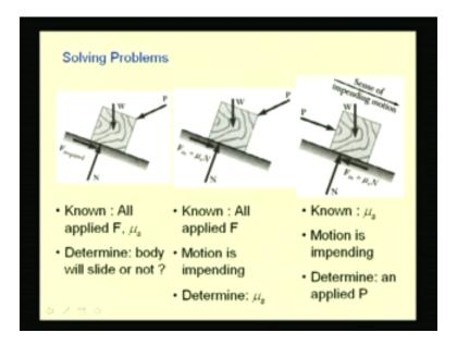
When we solve problems involving friction, we may have different situations. That means we may be interested in certain cases to determine the coefficient of friction that is needed, or in some other cases we may be interested in finding the required force in order to cross a required motion, etc.
