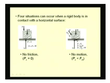
In the entire region where the friction is developed, right from the body which is in equilibrium and which is static to the point when it impends to move, the behavior can be divided into four
