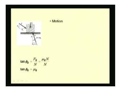
When the motion starts, we know that this reaction drops that means its inclination comes down because the horizontal component of the force reduces and becomes the kinetic-frictional force  $F_k$  which is less than the applied horizontal force. The angle of this resultant with the normal is equal to the angle of kinetic-friction  $phi_k$ . This angle  $phi_k$  is related to the coefficient of friction  $mu_k$  by considering these force relations.
