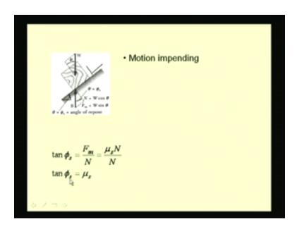
Here we see a block in an inclined plane. So the horizontal component or the component of the weight along the plane, if we take these as our coordinates, then the component of this weight along this plane tends to move this object in the downward direction. So a frictional force develops which acts against this force which is this  $F_m$ .
