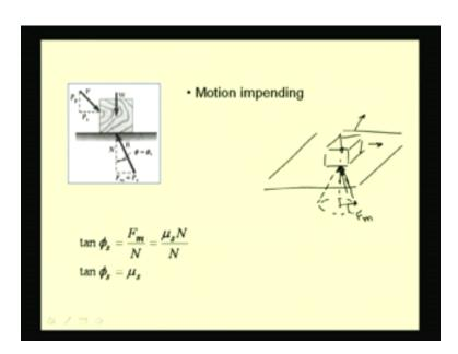
If the motion is impending then this angle is equal to  $phi_s$ , what we call as the angle of static-friction, in which case the developed frictional force is equal to the maximum limiting force that is  $F_m$ . So we have  $tan\ phi_s$  as F by N.
