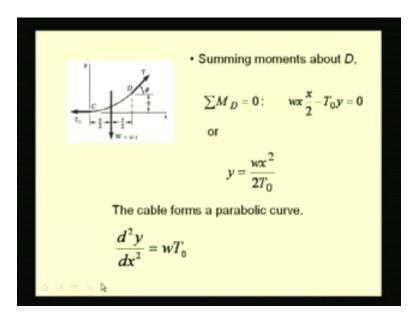
Let us sum the moments of these forces about this point D. We have this vertical force wx having a momentum of x by 2 which causes a counter clockwise moment; so it is positive. So we have wx into x by 2. The moment of this force  $T_0$  is a clockwise moment; so we have a negative moment minus  $T_0$  times y which is the momentum of this force  $T_0$  about this point D.
