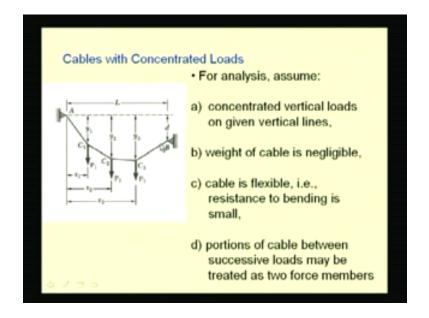
Here you see an example of a cable that supports concentrated loads. The cable is supported at A and at B and carries some concentrated loads say  $P_1$ ,  $P_2$ ,  $P_3$ , etcetera at various locations  $C_1$ ,  $C_2$ , and  $C_3$ . These loads as well as their horizontal spans are known. The interest is to know these y coordinates, that is, the shape the cable will take once these loads are being applied to this cable.
