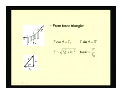
Let us construct the free body diagram and from this free body diagram write down the equations relating these forces. One graphical method of solving of the equilibrium particularly, in case of two-D is using the force polygons or force triangles. Here you see that method applied. You mark these forces  $T_{0}$ , T and W. For equilibrium to exist the sum of all these forces has to be 0. So that means they have to form a closed polygon where the ends of the vectors have to meet.
