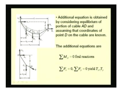
Let us assume that we know the coordinate of this point D on the cable. It could be any point either in this segment or in this segment. If we know this, let us draw the free body diagram of one portion of the cable: that is, either  $AC_1D$  or  $DC_2C_3B$ . Let us consider this portion  $AC_1D$  and draw the corresponding free body diagram.
