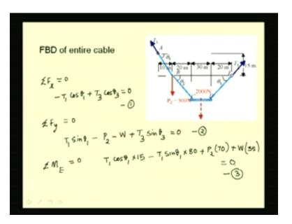
Let us draw the free body diagram of the complete cable. This figure shows the free body diagram of the complete cable. At E we have this end reaction which is equal and opposite to the tension that occurs in this portion DE that is  $T_{3}$ , so that is what the end reaction has been marked as  $T_3$  in the opposite direction.
