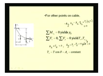
Let us consider this section  $AC_1C_2$  and draw the free body diagram. Since we have determined both  $A_x$  and  $A_{y}$ , we know the tension that will be occurring in this segment, that is,  $AC_1$ ; so we do not need to consider the free body diagram of the portion  $AC_1$  again. But now we do not know the tension in this segment, that is  $C_1 C_2$ ; so we take this segment and consider the free body diagram.
