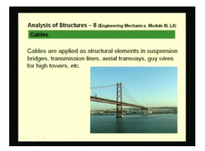
We will see how to analyze the internal forces in cables in this lecture. The cables, being flexible elements, are subjected to tensile forces only because they cannot resist any compressive force and they cannot also take any bending moment.
