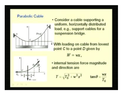
Let us consider few examples of uniformly distributed loads on cables. One, we call it as a parabolic cable because the shape of the curve taken by the cable is a parabola. This occurs when the cable is loaded uniformly along the x direction. This kind of a situation can be approximated for cables which support the bridges.
