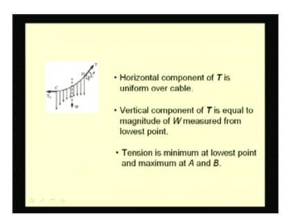
If we move this point along the cable to any other location, the tension in the cable changes, but we see that the horizontal component of this tension T which is equal to T cos theta has to be equal to the tension at this point C throughout the length of the cable. So the horizontal component of this tension force T remains constant and equal to  $T_0$ .
