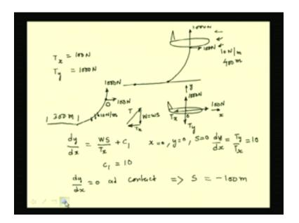
Let us solve one example problem. Consider a blimp which is tied to a cable such that certain portion of the cable is lying on the ground and certain portion of the cable is hanging. The weight of the cable as 10 Newtons per meter and the length as 400 meters is given. As this blimp is flying, it is developing a forward thrust of 100 Newtons against the air resistance and it is developing a lift of say 1000 Newtons.
