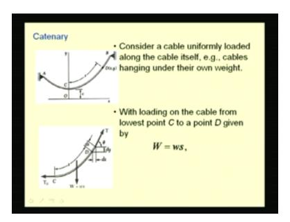
Let us consider now the cable which is loaded uniformly along its length because in all the previous cases we have not concentrated on the effect of the weight of the cable itself. The weight of the cable acts along the length of the cable and in the previous discussions we have not considered the same, so let us see how the shape of the cable changes if we consider the self-weight of the cable.
