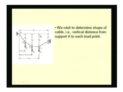
Our interest is to determine these vertical coordinates of the point of loading or in other sense the shape of the cable.
