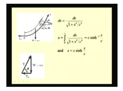
We integrate it between this point and the point of our interest. So the integral is 0 to s  $d_s$  by root of 1 plus s square by c square which is equal to c times of sin hyperbolic inverse s by c. Rewriting this, we have s equal to c sin hyperbolic of x by c. This equation relates the horizontal coordinate x to the path coordinate or the length of the cable s.
