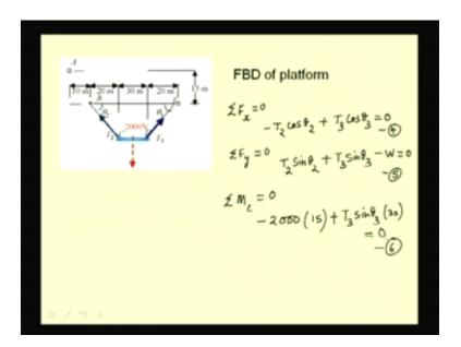
Here you see the free body diagram of the platform CD. The unknowns are the tension occurring in the portion DE and the portion BC which is  $T_2$ . From this free body diagram for the equilibrium, we can write three equations, two force summations and one moment equation.
