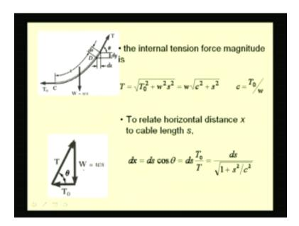
The internal tension force T's magnitude can be related to the vertical force w and the horizontal force  $T_0$  or the tension at C as T equal root of  $T_0$  square plus w square s square from the force triangle. If we write  $T_0$  by w as c then this can be rewritten as w times root of c square plus s square, where c is the ratio of this horizontal tension to the uniform weight w. So this is obviously from this force triangle.
