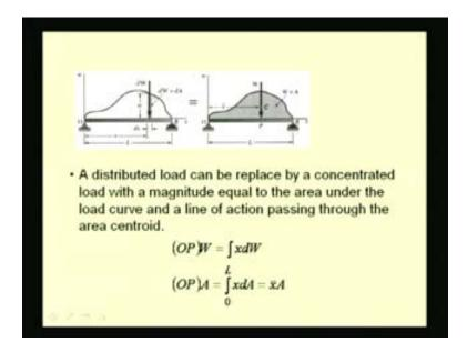
If you want to represent this distributed load by a concentrated load, so that we can use the shear force and bending moment drawing procedures of concentrated loads for the distributed loads also. So in order to do that we have to find an equivalent concentrated load for any given distributed load.
