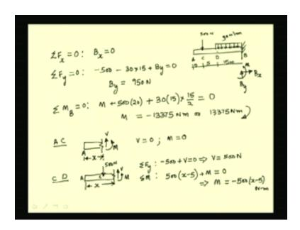
Let us see one example. Let us consider a beam which is cantilevered at B and supporting a point load of say 500 Newtons at C and supporting a uniformly distributed load up to point D from B. The dimensions are known and all the dimensions are in meters.
