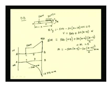
Let us consider the portion DB and draw the free body diagram of the same. We have a concentrated load of 500 Newtons at C and from the point D, we have this uniformly distributed force of 30 Newtons per meter.
