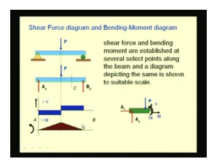
Today, we will continue with the discussion on the internal forces and see how to depict these forces as a diagram. We have the shear force diagram and the bending-moment diagram depicting the shear forces and the bending moment, which are the predominant internal forces in a beam, along the entire length of the beam for a particular loading and support condition.
