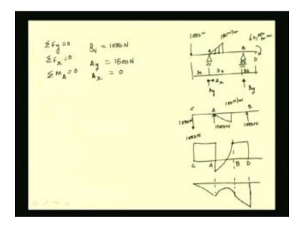
Let us say we have a beam with a pin reaction at A, the roller reaction at B, the uniformly varying load of say 100 Newtons per meter and a point couple at say the point D which is equal to 60000 Newton meter. Various dimensions are 30 meters, 30 meters and 30 meters
