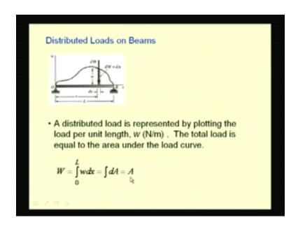
If the beam is loaded with uniform loading like the loading pattern shown in this picture, we have this beam OB which has a loading pattern defined by this load curve.
