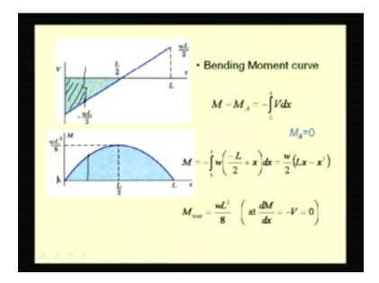
Here we see that the shear force is linearly varying. The area under this curve can be found out and the bending moment at any section, say a section at this point, is equal to the negative of the area under the shear force curve, that is, the area of this portion and that will be the bending moment at this section.
