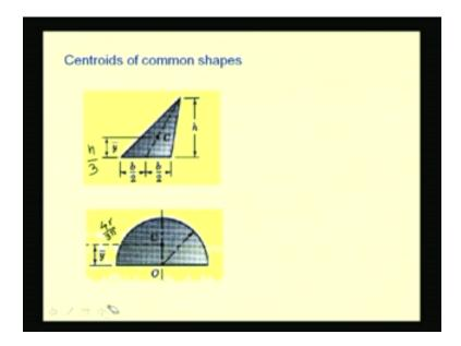
For common shapes we know the location of centroids. Like for this triangular lamina, the centroid lies along the angle bisector and at a distance of h by 3 from the base. Another lamina is shown; here, from this geometry we say that the centroid lies along one of the diametrical lines and at a distance of 4r by 3 pi, if r is the radius.
