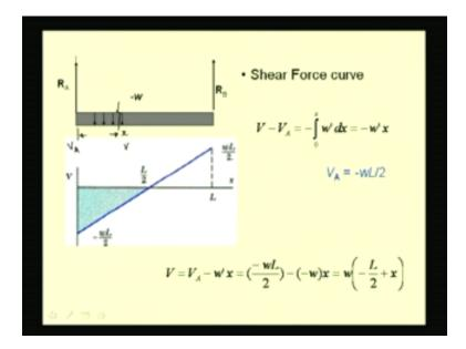
Now let us see how to determine the shear force curve from this loading curve. For the points where we have concentrated loads, we have to use the algebraic relations to find the shear force. So we can find the shear force at A.
