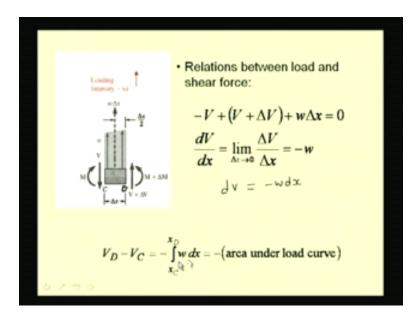
Let us first derive the relation between the load and the shear force. For equilibrium of this element CD, the total forces have to be 0 from which we get minus V, the force at C, plus the upward force V plus del V at D plus the upward forces which are applied, that is w delta x, on this incremental beam portion to be equal to 0.
