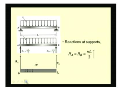
Let us take a beam AB with an uniform loading of w Newtons per meter for the entire length of the beam L. First, we determine the end reactions and it can be quickly found that these reactions have to be equal to half of the total load. The total load is area under the load curve which is w times of L, so we have the reactions at A as well as B as wL by 2.
