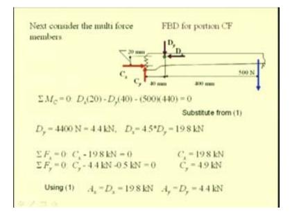
This is the free body diagram. At C, we have a reaction which is both unknown in magnitude as well as in direction; so we represent that by  $C_y$  and  $C_x$ . two components. At D, we have the joint forces that is  $D_y$  and  $D_x$ , which has been accounted for in the earlier free body diagram and at F, the plumber applies a force of say 500 Newtons.
