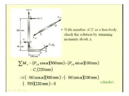
Now we move to the next multi force member that is ACE and we draw the free body diagram of this member. We have this pin reaction at A; so the two unknowns are which have been determined earlier from the free body diagram of the complete frame are shown here. The two reactions  $C_x$  and  $C_y$  have been determined from the free body diagram of the previous multi force member. The force from this two force member ED,  $F_{DE}$  again has been found from the previous free body diagram.
