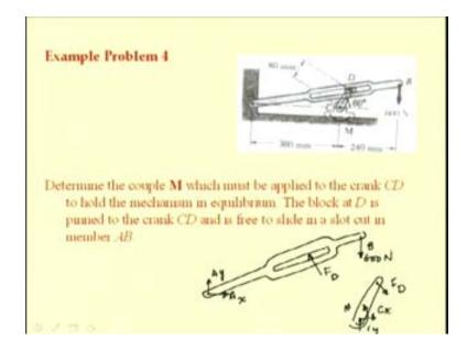
Let us consider another example. We will just consider how to draw the free body diagrams. Later on, one can proceed the way we have illustrated in the earlier example. Here, you see a mechanism which has a slotted arm ADB and a crank CD. We are interested to know the moment that has to be applied on to this crank at C, in order to support this load of 600 Newtons.
