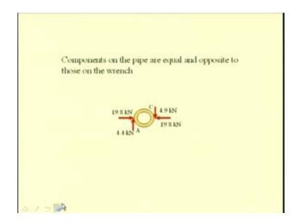
In order to know the forces on the pipe, they will be the equal and opposite forces that are being applied at A and C. We have these forces 19.8 kilo Newton, 4.4 kilo Newton, 4.9 kilo Newton and 19.8 kilo Newton force being applied on to the pipe.
