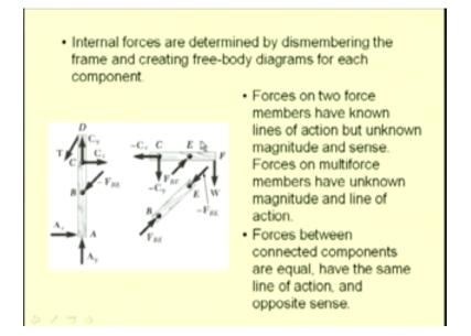
Now, in order to analyze the forces that act at various points of these interconnected bodies, we have to dismember and construct the free body diagram of each of the constituent members; both multi force as well as two force members and solve the resulting equilibrium equations.
