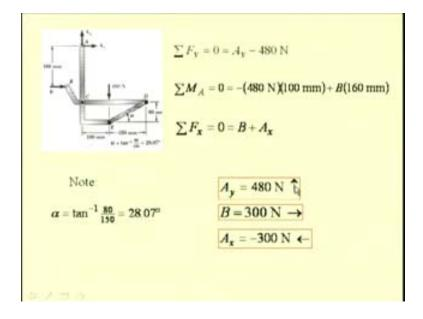
Once we determine the supports using these equations, we can proceed further to determine the internal forces. These are the three equations that result from the free body diagram of this complete frame. The force summation about the y axis when equated to 0 predicts the force  $A_y$ ; because we have  $A_y$ , the vertical component of reaction at A and the 480 Newton which is downward so —480 Newton equated to 0 can be used to find the force  $A_y$ .
