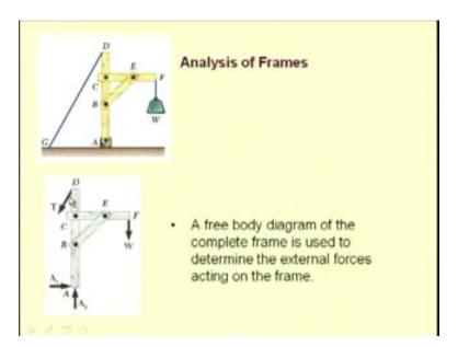
We will take the same example to illustrate the analysis procedure. In order to proceed, first we have to determine the external reactions for the frame under the given loading. We have this frame ABCDEF, with applied load at F, and reactions at A as well as at D. Let us construct the free body diagram.
