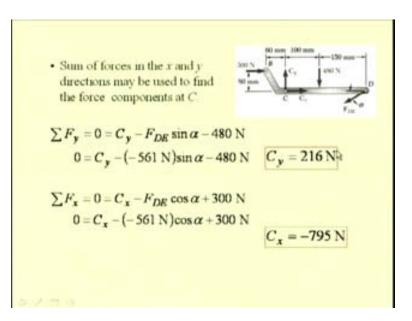
Before moving on, we can determine the other two reactions that are  $C_x$  and  $C_y$  from the two force summation equation. Summing the vertical components of the forces, we can determine this force  $C_y$  as 216 Newton. Summing the horizontal component of forces we know the horizontal component of the reactions  $C_{x_i}$  the same has been determined as 216 Newton and minus 795 Newton.
