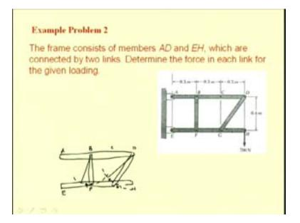
Let us see an example. Here you see a frame ABCDEFGH. The member ABCD is connected to the member EFGH by two, two force members: one is this BF and other is this GD. This frame is connected by pins at A as well as at E and we have an external load of 700 Newton applied at H. First, let us see whether the frame under consideration is a rigid body or not.
