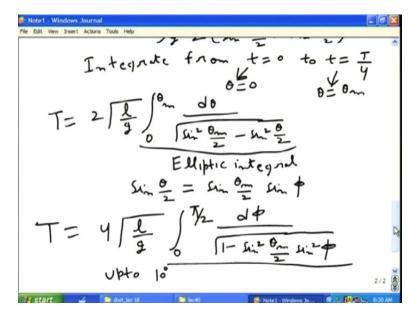
Integrate from t is equal to 0 to t is equal to T by 4. Then, at t is equal to 0; theta is equal to 0 and at t is equal to T by 4, where capital T is the time period, theta is equal to theta m. Doing this, we obtain T is equal to 2 under root 1 by g 0 theta m d theta by sin square theta m by 2 minus sin square theta by 2. This cannot be further simplified. So, this integration cannot be determined in an exact manner. It can be determined numerically.
