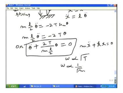
The governing equation for this case is m, this is the mass and this will be equal to 1 by 2x is equal to 1 by 2theta double dot. This is basically x dot, because x double dot x is equal to 1 theta. So, x double dot is equal to 1 theta double dot. Therefore, equation becomes m 1 by 2 theta dot dot. Now this is equal to T. This tension of this string is T. Assume that there is no change in the tension. Tension is directed here, T sin theta. So, it will be minus 2T sin theta.
