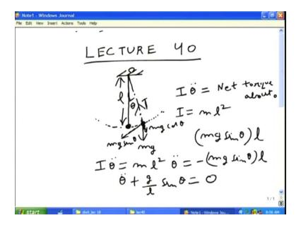
We have already discussed simple pendulum. This is a small bob attached by a string and this is moving in a circular path. This is the next position and that can be like this. This angle is theta.
