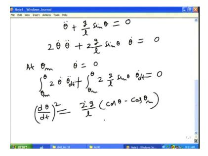
Let us integrate this equation between position of maximum amplitude, maximum displacement that is the last point of the amplitude. Now, theta will be the time. So, at theta m, let us say, theta m is the maximum displacement; so at theta m, theta dot must be 0. Integrating it, theta m theta 2 theta dot theta double dot. So, initial position is theta m and final position is any arbitrary theta plus theta m theta 2g by l sin theta into theta dot is equal to 0.
