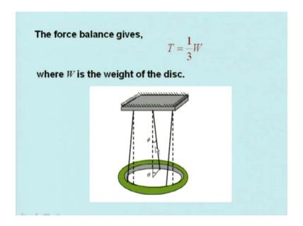
This force balance gives, T is equal to 1 by 3 W. Disc is acted by a gravity force W, and then there is a tension T in the strings which is 1 by 3 W. W is the weight of the disc. We can provide a small twisting in this plane of the disc. That means, disc remains in its own plane, but this radial point, radius moves to another point that is theta. Therefore, these strings get inclined. So, this is phi.
