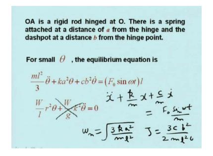
OA is the rigid rod hinged at O. There is a spring attached at a distance of a from the hinge, and the dashpot at a distance b from the hinge point. So, dashpot is that. For a small theta, the equilibrium equation is ml square by 3 theta double dot plus ka square theta. ml square by 3 is the mass moment of inertia of the cylinder rod about point O.
