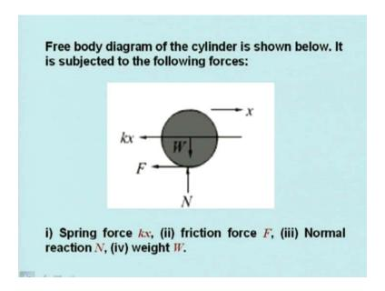
Now, make the free body diagram of the cylinder which is shown here. I have shown the cylinder. Make the free body diagram. What are the forces? Let us discuss the forces coming on the centre.
