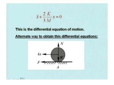
Therefore, x double dot plus 2 by 3 M. x is equal to 0, because here, this will be 3 by 2 Mx double dot plus kx equal to 0. Compare this equation with the spring-mass system, where we had Mx double dot plus kx equal to 0. We are having 3 by 2 Mx double dot plus kx. Therefore, effective mass is actually more. Therefore, x double dot plus 2 by 3 km plus x equal to 0. This is the differential equation of the motion of a cylinder held by the spring.
