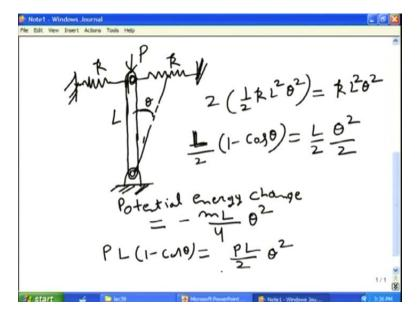
If you take a rod and there is a spring attached here, k and this spring is attached on this side as well this is k, this is P and this is L. Let a rod of mass m and length L is restrained in the vertical position by two identical springs having spring constant k, a vertical load P acts on the top of the rod. This is acting if given a small displacement theta to the rod, one spring compresses by amount L theta.
