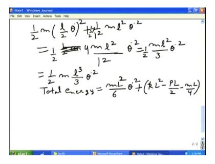
So, kinetic energy of the rod is equal to half m l by 2 theta square plus 1 by 2 ml square theta dot square, or basically it will come l square by 4 and this is 1 by 12. It is I theta square, because this will become equal to half m l square by 12 and this is 4. So, you can take 4 common and this becomes l square ml square by 12. This is 3 plus 1, 4 ml square by 12 theta dot square or ml square by 3 theta dot square into half 4 ml square.
