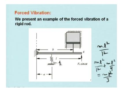
Now, we have talked about the free vibration problems. Let us go to the forced vibration problem. An example of a forced vibration of a rigid rod is like this; this rod is hinged at this point and an excitation force  $F_0$  sin omega t is provided at point A. Dashpot is at a distance of b. This distance is l. This is the spring. Here, the spring stiffness is k. This is a, this is b. Now, this is d. This is a dashpot, linear dashpot.
