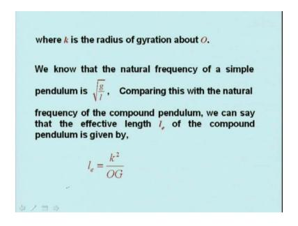
We know that the natural frequency of a simple pendulum is square root g by l. Comparing this with the natural frequency of the compound pendulum, we can say that the effective length  $l_e$  of the compound pendulum is given by  $l_e$  is equal to k square by OG, because in this expression, this is compared with under root g  $l_e$ . Therefore,  $l_e$  square  $l_e$  is k square by OG.
