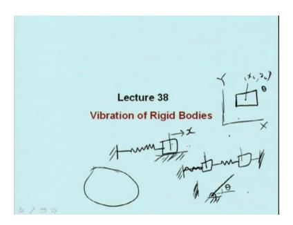
We obtained only one dimensional equation. We had x, position of the mass or that particle is described only by x. So, independent coordinate is x; therefore, this is a single degree of freedom system. If I would have kept like this, suppose there are mass and this was the spring, another spring, another mass; Then this would have become 2 degree of freedom system, because I need to tell the position of this mass, then I need to tell the position of another mass, so, 2 degree of freedom system.
