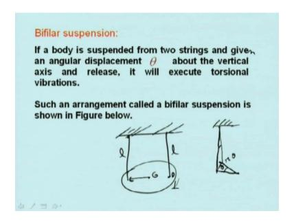
We discuss bifilar suspension. If a body is suspended from two strings and given an angular displacement theta about the vertical axis and released, it will execute torsional vibration. Such an arrangement is called bifilar suspension. I am drawing the figure here. A bifilar suspension will be like this and it is a disc type of thing. It is how, a string is attached here.
