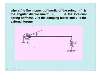
Let us take a rod here. It is fixed here. A torsional spring is with this. When the rod rotates by theta then a restoring moment is developed; that is  $k_t$  times theta. That restoring moment will be  $k_t$  times theta and this side, we have kept a linear spring, whose spring constant is k.
