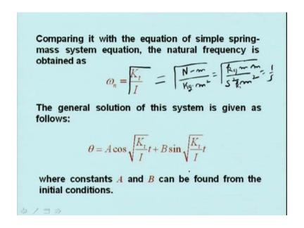
Therefore, omega<sub>n</sub> is natural frequency and is obtained. omega<sub>n</sub> is equal to under root  $K_t$  by I.  $K_t$  has the unit of Newton meter. Let us see the units here; Newton meter kg meter square and Newton is kg meter per second square. So, you have second square then one meter was already there, meter meter square. So, meter meter gets cancelled it becomes and this is kg. So, you get 1 by s. So, omega<sub>n</sub> means its unit is second inverse.
