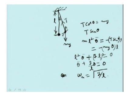
Simple pendulum consists of a string. With that, you attach a small ball. It can be treated as particle. The entire mass is concentrated here and this is l. If you displace it here, there is no spring here, but if you displace it there, its potential energy rises and gravity tries to pull it to another lowest position. So, at this moment, there is a gravitational pull that is mg and then you
