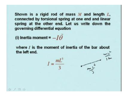
Inertia moment is minus I theta dot dot. I is the moment of inertia of the bar about the left end and this is given by m L square by 3. You have a rod and its moment of inertia, uniform slender rod, its moment of inertia about this point is m L square by 3. About its cg, it is m L square by 12 so I equal to m L square.
