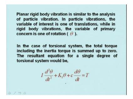
In this case, the total torque including the inertia torque is summed up to 0; that is D D'Alembert's principle, or we can say that we can apply the Newton's law generalized to that
