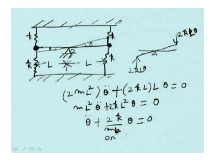
Let us try to solve some other problems. If there is a pivot here and one rod is fixed. At the end of the rod, I took two small balls and their masses maybe m. Then, here you attach, this is the upper that force one right and here another fixed wall and here you attach a spring like this. Assume that, this figure I have drawn is in a horizontal plane. So, gravity effects are not there. It is in a horizontal plane, so, it vibrates.
