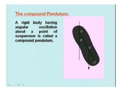
Discussing about compound pendulum, in compound pendulum, mass is not concentrated at one point. In fact, it is distributed. This is the compound pendulum, shown. A rigid body having angular oscillation about a point of suspension is called a compound pendulum. Here, the mass acts through the center of gravity.
