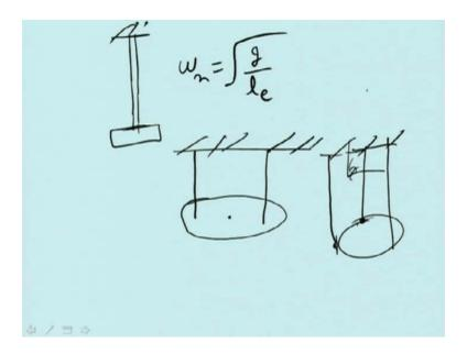
First we took up the case in which a torsional spring was put. After that, we have discussed the case of a disc suspended from a rod or shaft. When we twist it, the shaft gets twisted and due to elasticity, it tries to come back to its position. Therefore, it has some equivalent stiffness. We have discussed that case also.
