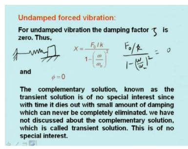
For undamped forced vibration, now undamped, one damping factor zeta is equal to 0. Thus, we get X is equal to  $F_0$  by k 1 minus omega by omega square and we get phi is equal to 0. There is no phase difference between the forcing function and the response. Then we are getting this type of expression. Here also, it is seen that if omega is very small then X is equal to, of course  $F_0$  by k, but if omega is very large then this X will approach 0 because of this term  $F_0$  by k. So, this
