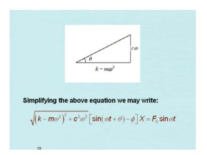
We assumed that the force was  $F_0$  sin omega t but our displacement was sin omega t minus phi; that means, there was a phase difference between two. So, this gives the idea about the phase difference.
