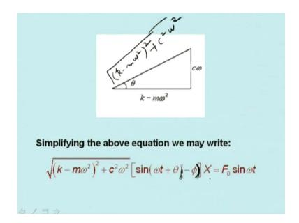
If we compare the right and left hand side of this thing, sin omega t, this has to be equal. So, omega t plus theta minus phi should be equal to 0.
