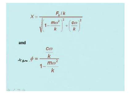
We can write X as  $F_0$  by k divided by k. So, 1 minus m omega square by k whole square plus c omega by k whole square and c omega by k 1 minus m omega square by k. It is to be noted that  $F_0$  by k is the static deflection of the spring under the action of that force  $F_0$  k. Maximum amplitude of the force is  $F_0$ . So, if you apply maximum force then you will get the static deflection as  $F_0$  by k.
