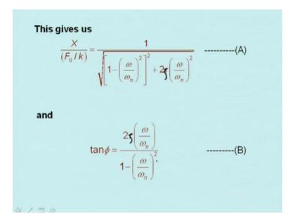
This gives us X divided by  $F_0$  by k is equal to 1 under root divided by under root 1 minus omega by omega<sub>n</sub> Whole Square whole square plus 2zeta omega by omega<sub>n</sub> whole square. This is also zeta. This tan and tan phi is equal to 2zi omega by omega<sub>n</sub> 1 minus omega by omega<sub>n</sub> Whole Square.
