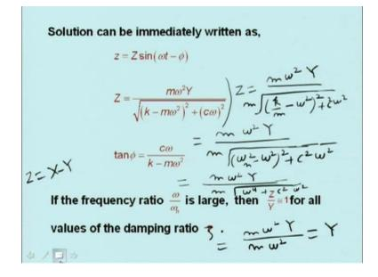
Its solution can be immediately written as z is equal to Z sin omega t minus phi. Because this type of thing we have already done. This is like a force. Instead of the force  $F_0$  sin omega t, we are having m omega square Y. So, m omega square Y is like a force. So, z is equal to Z sin omega and Z is equal to m omega square by Y under root k minus m omega square whole square plus C omega square and tan phi is equal to C omega k minus m omega square.
