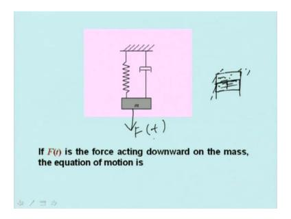
Then we represent this system in which viscous damping, viscous damping means there is damping; that means, resistance is proportional to the velocity, but in the negative direction minus cx. So, that means acceleration is proportional to this is force, damping force is proportional to F(t). Take the mass then represent by a spring. Then again, we have a dashpot.
