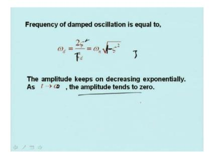
Frequency of damped oscillation is equal to, omega<sub>d</sub> is equal to 2 tau divided by  $T_d$ . This is  $T_d$  that is omega<sub>n</sub> 1 minus tau square. That is not tau. This is basically zeta. The amplitude keeps on decreasing exponentially as t tends to infinity, the amplitude tends to 0. So, that way, you know damp motion will take place and this is how it will be covered.
