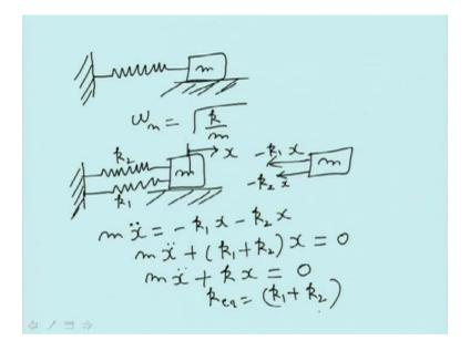
This is the spring mass system, here omega<sub>n</sub> is equal to under root k by m. What happens if we put two springs here? What type of equations we will get?
