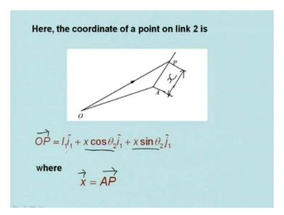
Now, about the point O, the coordinate of point on link 2 is suppose P, so position vector OP is  $l_1$   $i_1$  plus x cos theta<sub>2</sub>  $i_1$  plus x sin theta<sub>2</sub>  $j_1$ , where basically x is equal to AP. This is x. In this figure, this is x. We want to find out the position vector of point P that means position of point P with respect to O. So if we differentiate this position vector twice, we will get the absolute acceleration of point P. That is what we need.
