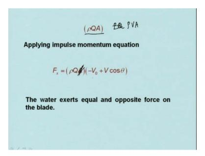
Rho QA is the rate of mass coming on that; Q is the discharge, A is the area and rho is this one. We can say Q or it should be rho times  $V_A$ . Then applying momentum equation in this equation, we have rho Q and this is minus  $V_0$  and plus V cos theta, that is the change in the momentum. So, Vcos theta minus  $V_0$ , that is  $F_x$ . So, water exerts equal and opposite force on the blade. There is no net vertical force in this problem because of symmetry.
