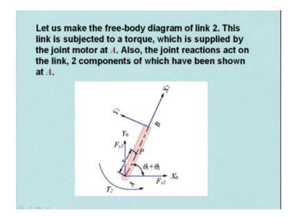
We can make the free body diagram of link 2. Now, this is the link 2. Here, I have shown the axis system also. One fixed axis is like this, X and Y here. Then you have  $X_1 Y_1$  that is  $X_1$  is along the link 1 and  $Y_1$  is perpendicular to that one. So it is a moveable coordinate system that is attached at point 1 and similarly  $X_2 Y_2$  is like this; that along this and this is this thing.
