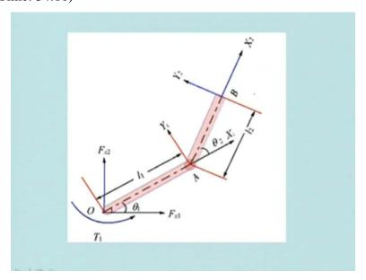
We are considering the free body diagram of the links together. We could have drawn the free body diagram of only the link 1. In that case, the joint reactions will be coming at join A. Those are unknown to us, so we do not want to find out. That is why we are doing like this and in this case, you are showing that joint reactions  $F_{x1}$   $F_{x2}$  here and then torque  $T_1$  acting.
