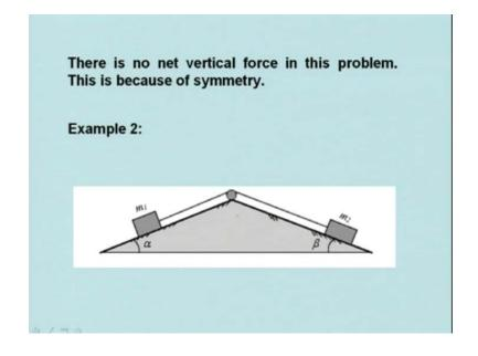
Now example 2 of interconnected bodies, suppose two bodies are acting here. This is  $M_1$  and this is  $M_2$  and they are put on the inclined plane. This is alpha and this is beta, angle inclined with this.
