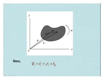
For example, this is the situation. You have body. This is the axis system; G is the mass center and it is rotating with angular velocity omega, and  $rho_i$  is the distance of the mass from this and this is  $r_i$  and this is  $r_G$ . We have the absolute velocity term here  $m_i$   $V_i$ , but  $rho_i$  is the position vector of the particle about the center of the mass. Then you have  $V_i$ ; that means, velocity of the particle is r dot i is equal to rho dot i plus r dot G.
