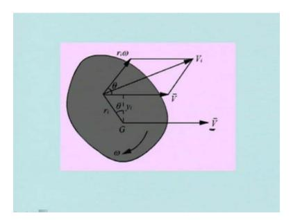
This type of situation is there. See this body. It is rotating and at the same time, the mass centre G is going with a velocity of V bar. It has been indicated. So, any particle on the body that is at a
