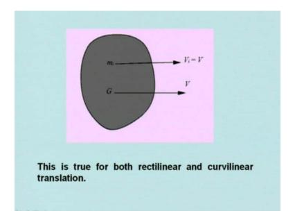
Here, the velocity of the mass center G is like this and velocity of any other particle is also same. So,  $V_i$  is equal to V. This is true for both rectilinear and curvilinear translation. No matter body is moving in a straight line or body is moving in a curved path, you have got the same type of relation. So, there is no problem in this.
