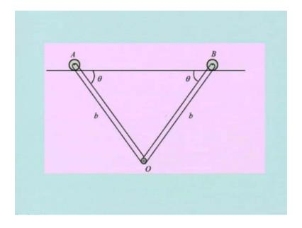
This is the problem. There are two rods here, this one of length B and these are rollers which are moving on a rail, and this is theta, this is theta and this is b and this is this one. At certain time two identical rods of length b have been arranged as shown in the figure. The rods are allowed to move in the vertical plane due to influence of gravity. Now, find out the acceleration of the rod at the instant depicted. It is this thing here that you have to find out the rod and this is.
