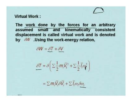
We come to the virtual work principle. We have studied that in statics. Here also, the same type virtual work principle can be used. The work done by the forces for an arbitrary assumed small and kinematically consistent displacement is called virtual work and is denoted by delta omega.
