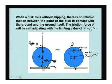
Let us consider this case. Here, this is the plane surface and the cylinder is rotating. This is the contact point C. From this, you are having a normal reaction N and then you are having the mass F. Then, there is a weight W. So, this is G, that mass center is G and this is W. You have some frictional force F. F actually will pass through this and then you may have some applied force
