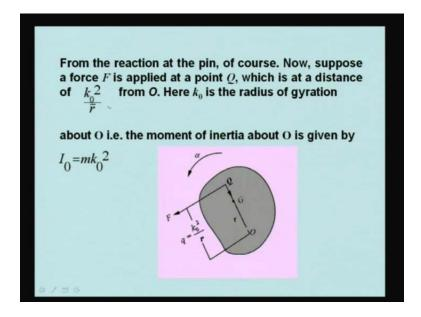
From the reaction at the pin you know that, because it is pinned at O we will get that. Suppose a force F is applied at a point Q, which is at a distance of Q is  $k_0$  square by r from O. Instead of that you know that is passing through G, if now we apply to pass through Q, where  $k_0$  is the radius of gyration about O; that is, the moment of inertia about O is given by  $I_0$  is equal to  $mk_0$  square, so this is given here.
