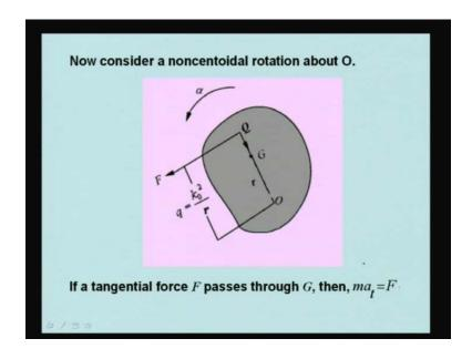
Consider a noncentroidal rotation about O. Like in this case, if we pass a tangential force through G, if the tangential force was passing through G then mass times at will be equal to F.
