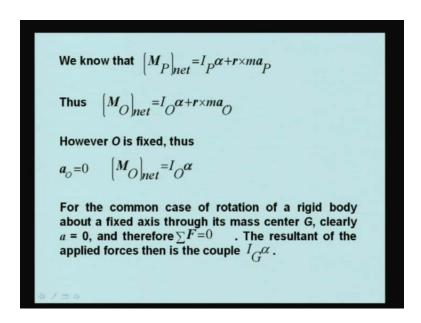
We also have discussed in this lecture, this equation that if you take any point P, say P is any point, then you get  $M_{Pnet}$  is equal to  $I_P$  times alpha plus r cross mass into  $a_P$ . Here,  $I_P$  is the moment of inertia of the body, second mass moment of inertia about the body. But it is about point P, and this is r cross m  $a_P$  here  $a_P$  is the acceleration of point P, not the point G, it is point P. So, we get this equation.
