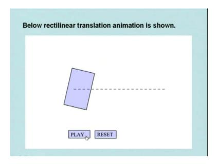
I am showing one animation for rectilinear translation motion. Here, any particle of the body is moving in a straight line. So, the particles here are moving in a straight line. Similarly, the particles here are moving in another parallel straight line. So this is the example of rectilinear translation.
