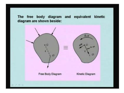
Now, free body diagram and equivalent kinematic diagram are shown here. Free body diagram shows the forces, externally applied forces and also the reaction forces passing through O. G is the mass center and then the kinetic diagram is this; mass times tangential acceleration, mass times normal acceleration is here and then you have got  $I_G$  times alpha.
