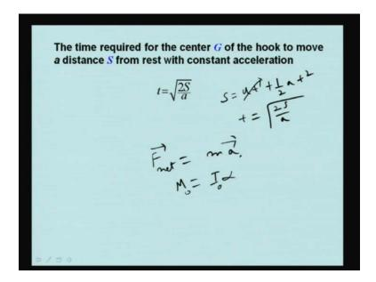
The time required for the center G of the hook to move a distance S from the rest with constant acceleration, obviously can be found by t is equal to under root 2 S by a, where 2 S is the distance because this is simple formula. S is equal to  $u_t$  plus half  $a_t$  square and this portion is being 0.
