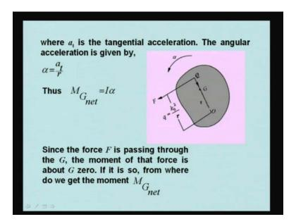
Where  $a_t$  is the tangential acceleration, the angular acceleration is given by alpha is equal to  $a_t$  times r. Thus, you will have  $M_{Gnet}$  is equal to I times alpha. Since the force F is passing through G, the moment of that force is about  $G_0$ . Now, if it is from where we do  $M_G$  net then from where, because we have to balance this  $M_G$  net is equal to I alpha, obviously we get it from O, because there are some points at that O.
