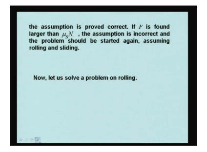
If F is found larger than  $mu_s$  times N then the assumption of pure rolling was incorrect. The problem should be started again. This time assuming that rolling and sliding. So, the equation and also the expression for force will change and F will now become equal to  $mu_k$  times N. Let us solve the problem on rolling.
