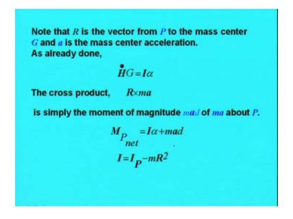
Therefore, R is the vector from P to the mass center G, and a is the mass center acceleration. We already know that H dot G is equal to I alpha and the cross product R cross ma is simply the moment of magnitude m times a times d of ma about aP where d is the perpendicular distance of acceleration vector from that point. Therefore,  $M_{Pnet}$  is equal to I alpha plus mad.
