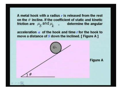
This will be like this. I have shown here an inclined plane; this is at angle theta and this is the metal hook G with a radius r that is released from the rest on the theta inclined. If the coefficient of static and kinetic friction is  $mu_s$  and  $mu_k$  then we have given that you determine the angular acceleration alpha of the hook and time t for the hook to move the distance of S down the inclined. So, this is shown here in the figure.
