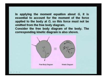
When you apply the moment equation about G, like you have to apply  $M_{G net}$  is equal to  $I_{G}$  times alpha, then always remember that you have to account for the moments of the all the forces applied to the body. That means, even you have to consider the forces, internal forces which are applied at O. When you make a free body you have to understand that there are some internal forces at O. These also have to be reaction forces and they have to be taken into account.
