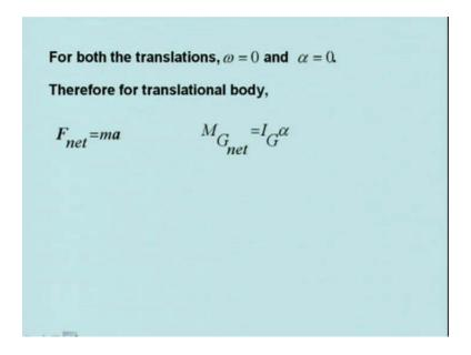
Therefore, for both translations omega is 0 and alpha is 0. So, for translation of a body,  $F_{net}$  then becomes equal to mass times acceleration, because that was one equation. This is a vector equation,  $F_{net}$  is a vector and that is equal to mass into a and  $M_{Gnet}$  is equal to  $I_G$  times alpha. So,  $M_{Gnet}$  is this one and so alpha is 0. Therefore  $M_{Gnet}$  is 0, means if you take about the mass center that  $M_{Gnet}$  will be equal to 0.
