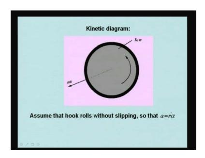
Then, we make the kinetic diagram. In that, we just show that mass times acceleration which is in the direction of inclined plane and that  $I_G$  times alpha. Now, assume that hook rolls without slipping, so that a is equal r times r alpha that equation is valid.
