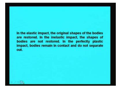
In the elastic impact, the original shapes of the bodies are restored. In the inelastic impact, the shapes of bodies are not restored. In the perfectly plastic impact, bodies remain in contact and do not separate out because there is nothing. No force is applied to decrease the area. Therefore, they keep moving with the common velocity and there is a plastic deformation. So, therefore they do not separate out. That is what happens in the perfectly plastic impact.
