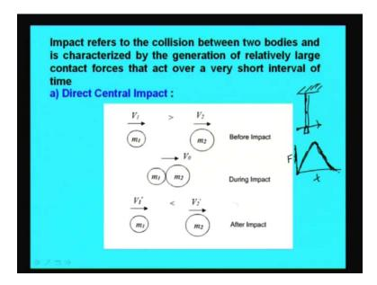
Let us see, what is the process of impact? Impact refers to the collision between two bodies and is characterized by the generation of relatively large contact forces that act over a very short interval of time. In collision, two bodies make contact and then large amount of contact force is generated. If body a, applies some force on body b, then body b also applies the same amount of force on body, a. There are mainly two types of impacts.
