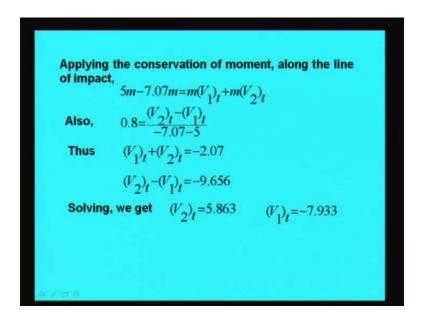
Then, you apply the conservation of momentum along the line of impact. So, 5 into mass, if mass is same. So, 5m minus 7.07m. In the beginning this velocity, this velocity is in opposite direction, so minus sign and is equal to  $m_1 V_1 t$  plus  $m_2 V_2 t$  normal, that is along the normal directions. Let us use the symbol n here. Also we have, coefficient of restitution is 0.8 given.
