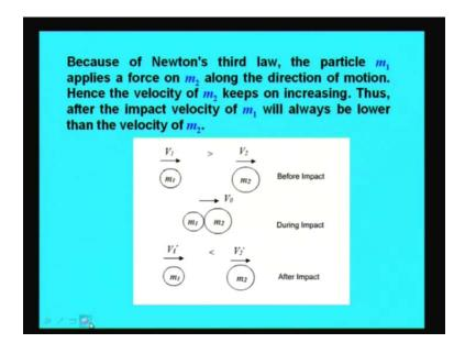
Because of Newton's law, the particle  $m_1$  applies a force on  $m_2$  along the direction of motion. Hence, the velocity of  $m_2$  keeps on increasing. Thus, after the impact, velocity of  $m_1$  will be always lower than the velocity of  $m_2$ . That is the point and it has to be noted out.
