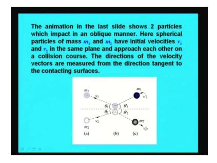
In this case, two bodies will make collision and the situation will be like this. There is a particle  $m_1$  and there is a particle  $m_2$ ; both are moving with the velocity  $V_1$ , this is moving with the velocity  $V_2$ , both may contact at this point, collide and after that they separate. So, you know that when they make contact, this is the normal direction and this direction is the tangential direction.
