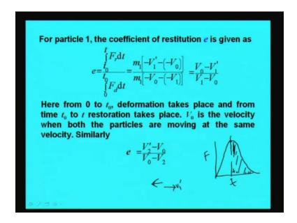
For particle 1, if we consider just the particle one, we can consider any one particle. We consider particle 1, the coefficient of restitution is given as e is equal to  $t_0$  to t. What is  $t_0$ ?  $t_0$  is that time at which bodies have started moving with the same velocity. The force has already reached maximum and this is like this. If bodies are deforming like this, this is time and this is F, this will be  $t_0$ .
