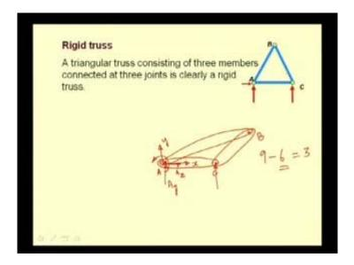
Before we proceed to analyze the structure, one has to understand what we mean by a rigid truss. So, here we see the most simplest form of a truss, that is, three elements AB, B C and AC connected at A, B and C and the truss is supported by a pin joint at A and a roller joint at C.
