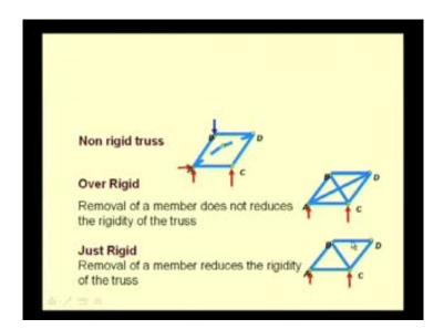
So, here we see an example of a truss which is not rigid. Here we see these members AB, BD, CD and AC, connected at A, B, D and C and supported by a pin joint at A and roller joint at C, but under the action of this external force at B, this truss element deforms, because sufficient number of degrees of freedoms have not been restrainted.
