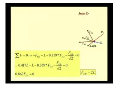
Now, that we have determined this force, we can move to this joint D. The various forces both internal as well as the external reaction and the externally applied load are shown in this picture. The direction cosines of various forces can be obtained from the geometry of the truss. And we have already determined the magnitude of this force in member CD and so only we have three unknowns, that is, the force in BD, force in the element ED and force in the member BA to be determined.
