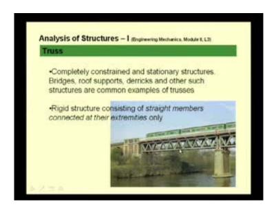
One such civil structure, which is known as trusses and we will see how do we analyze them, and determine the forces acting on its various members, in order to predict the performance of such structures. The picture accompanying the slide shows a typical truss used to support bridges; other examples are the roof supports, the derricks, the structures used to support the radio antennas and high voltage cables.
