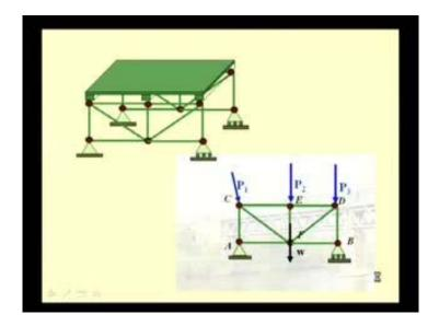
Let us see this example little more clearly. This picture shows a part of the bridge; so this is the bridge platform, which is supported by beams and these beams are supported by the trusses. So, here you see one plane truss in the front and another plane truss at the rear; plane trusses are trusses, whose elements lies in a single plane and their loading is also in the same plane. So, the problem can be analyzed as a two-dimensional problem.
