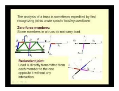
One kind of special loading is known as the zero force members and this picture depicts a truss element that is ABCDEF, connected by a roller at A, and by a pin joint at F, and various externally applied loads like F 1, F 2, F 3 at joints C, E and G.
