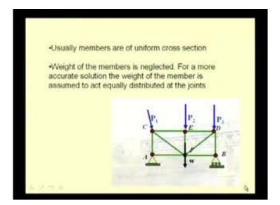
The weight of the members is negligible compared to the externally applied load, but for better analysis, we can consider the weight of the member to be equally distributed at their joints; let us say the weight of the members CE is equally distributed at joint C and joint E for an accurate analysis.
