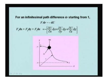
For an infinitesimal path difference dr starting from 1, F dot dr is equal to minus dU; that is  $F_x$  dx plus  $F_y$  dy plus  $F_z$  dz is equal to minus delta U by del x dx plus delta U by del y dy plus del U by del z dz.
