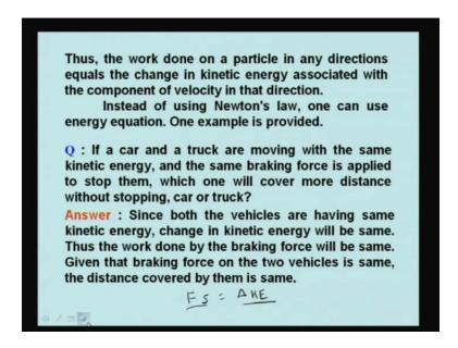
Thus, the work done on a particle in any directions equals the change in kinetic energy associated with the component of velocity in that direction. This is very important because we can find out the velocity components by using the work and kinetic energy equation. One example is provided. If a car and a truck are moving with the same kinetic energy and the same breaking force is applied to stop them, which one will cover more distance without stopping, car or truck?
