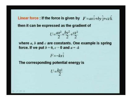
Linear force: if the force is given by F is equal to ax i plus by j plus cz k, then it can be expressed as the gradient of U is equal to ax square by 2 plus by square by 2 plus cz square by 2, where a b and c are constant. If you take the gradient of U, this becomes ax i plus by j plus cz k.
