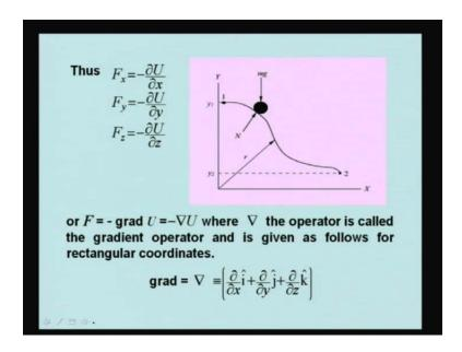
Thus  $F_x$  is equal to minus del U by del x,  $F_y$  is equal to minus del U by del y,  $F_z$  is equal to minus del U by del z, or F is equal to minus gradient of U, where U is a scalar field and this is indicated
