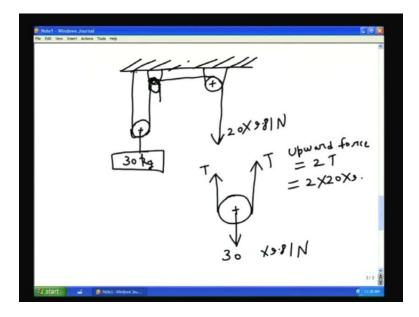
Consider pulley mass system. This is a pulley, where this string is passing. Then another pulley then this string goes like this and this is going here. If a force of 20 into 9.81 Newton is applied, a mass of 30 kg is suspended from here. We have to find out the acceleration of 30 kg mass, when the cart is being pulled by 20 into 9.81 Newton force. We neglect friction and the mass of the pulley and then make the free body diagram of 30 kg mass as well as pulley attached to it.
