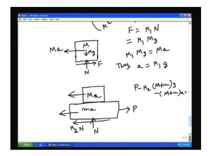
Now, from the free body diagram of the crate plus cart in this inverse m, this is the cart M, this is force N,  $mu_2$  N. P this is P minus  $mu_2$  M plus  $M_g$  minus M plus M into a equal to 0.
