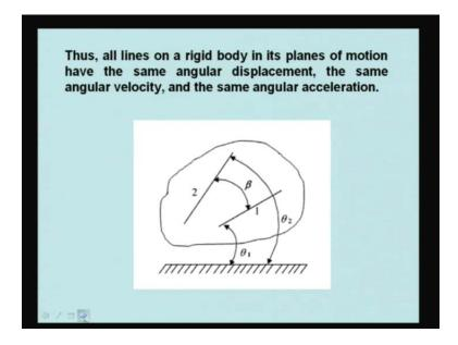
Thus, all lines on a rigid body in its plane of motion have the same angular displacement, the same angular velocity and the same angular acceleration.
