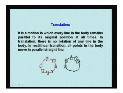
Translation: It is a motion in which every line in the body remains parallel to its original position at all times. There is no rotation of the lines in the body. In translation, we have two types of translation: one is rectilinear translation in which all points in the body move in parallel straight line. Then we have curvilinear translation in which is the points do not move in parallel straight lines, but they move in parallel curves. Now, the body may move in a circular path also.
