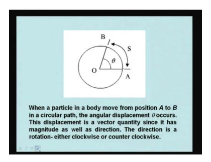
When a particle in a body moves from position A to B in a circular path like this, the particle A has gone from A to B, the angular displacement theta occurs. This displacement is a vector
