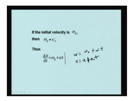
If the angular velocity is  $omega_0$  then at time t is equal to 0, omega is equal to  $omega_0$ ; thus,  $C_1$  is equal to  $omega_0$  is equal to  $C_1$ . Thus, d theta by dt is equal to  $omega_0$  plus alpha t, or omega is equal to  $omega_0$  plus alpha t. This is the same way as you get equation of motion; v is equal to u plus at.
