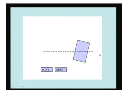
See this animation. Here, the body is moving in parallel straight line. If we know the velocity of any one point on the body, we have known the velocity of whole body; because, all the particles are moving in the same way. So, the velocity of all the particles is same in direction as well as magnitude in this case.
