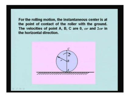
For the rolling motion, suppose the body is undergoing rolling motion then the instantaneous center is at the point of contact of the roller with the ground. It is in contact with the ground. The velocities of points A, B and C are 0, omega r and 2 omega r in the horizontal direction. If the body is not undergoing pure rolling, that means there is a slipping also; in that case, A will not have a 0 velocity and therefore, A will not be called instantaneous center.
