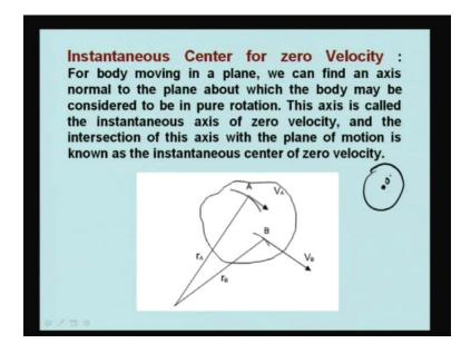
Now, we will discuss another point, the instantaneous center of zero velocity. For a body moving in plane, we can find an axis normal to the plane about which the body may be considered to be in pure rotation. We can always find out a point about which body can be considered to be in pure rotation. This axis is called the instantaneous axis of zero velocity. The intersection of this axis with the plane of motion is known as the instantaneous center of zero velocity.
