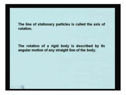
The line of stationary particles is called the axis of rotation. So, when the body rotates there is one axis of rotation. The rotation of a rigid body is described by its angular motion of any straight line of the body.
