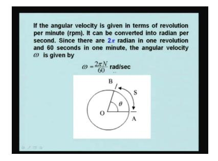
If the angular velocity is given in terms of revolution per minute that is rpm, most of the machinery items or motors will be specifying the revolution per minute; that is rpm; say a motor rotates 1450 rpm like that. It can be converted into radian per second. Since, there are 2 pi radian in 1 revolution and 60 seconds in 1 minute, the angular velocity omega is given by omega is equal to 2 pi N divided by 60 radian per second.
