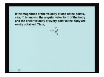
If the magnitude of the velocity of one of the points, say  $V_A$  is known, the angular velocity omega of the body and the linear velocity of every point on the body are easily obtained because omega will be equal to  $V_A$  by  $R_A$ . Once you have found that angular velocity of the point, then after that it is very easy to find out the velocity of any other point.
