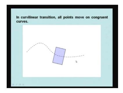
In curvilinear translation, all points move on congruent curves. This is an example of curvilinear translation. However, even in this case, the velocity is same for all particles. So, in this case the velocity may be changing, the velocity here may be small. Then, it is this thing. Body may be accelerating or decelerating that is a different issue but velocity of one particle is same as the velocity of any other particle of the body. So, this is an example of that curvilinear translation.
