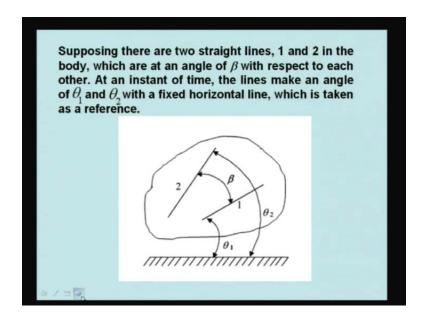
Any straight line, why we say any straight line? Supposing there are two straight lines; 1 and 2 in the body which are at an angle of beta with respect to each other. A body line 1 is there and line
