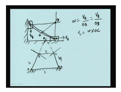
If you are having a mechanism like this, there is a slider here; join this by pin joined with a link. This one, this is slider A and this is B. A, can slide on the horizontal floor and B slides on the other, this perpendicular.
