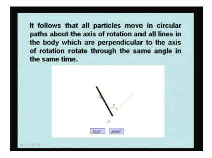
It follows that all particles move in circular paths about the axis of rotations and all lines in the body that are perpendicular to the axis of rotation, rotate through the same angle, in the same time. Here, it is rotating. Now, all the particles are moving in a circular path. Also, all the particles which are in this line have rotated by theta. That means, if we consider this line, this is theta; this is also through the same angle in the same time.
