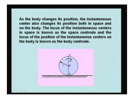
As the body changes its position, the instantaneous center also changes its position both in space and on the body. The locus of the instantaneous centers in space is known as the space centrode. If we draw the locus of the instantaneous centers in space that will be known as space centrode and the locus of the positions of the instantaneous centers on the body is known as the body centrode.
