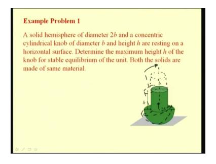
Here you have a solid which is composed of a cylindrical knob and a hemispherical base. The diameter of the hemispherical base is 2b which is twice the diameter of the cylindrical portion. The height of the cylindrical knob is h. We are interested to determine the maximum height h of
