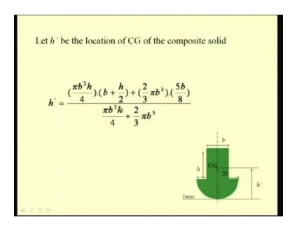
The location of the CG h prime is equal to the sum of these two quantities that is the volume of the cylinder into its location of the CG which gives the first moment plus the volume of the sphere times its location of the CG divided by the volume of the composite solid. From this expression, we get the expression for h prime. If we simplify this, we will get the required expression.
