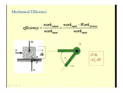
We have seen that the friction dissipates energy in the form of heat. We can define, now the efficiency of a mechanical system as the ratio of the available energy to the input energy where the available energy is nothing but the input energy minus the energy lost because of the heat dissipation due to the presence of friction.
