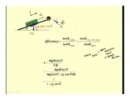
Let us write the virtual works that are involved for this virtual displacement and find this efficiency by writing that work output which is nothing but the work that is used to raise the load and work input is nothing but the work done by this force T for raising this load.
