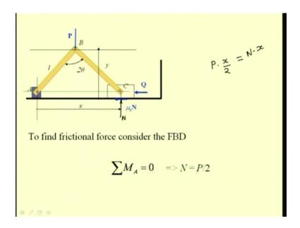
In order to find this frictional force that is  $mu_k$  N which is the unknown force, we have to consider the free body diagram and solve by considering the equilibrium equations. We have already seen that when we have friction in the system, we have to go by our traditional methods of equilibrium to solve for the unknown because the virtual method work does not give any additional advantage.
