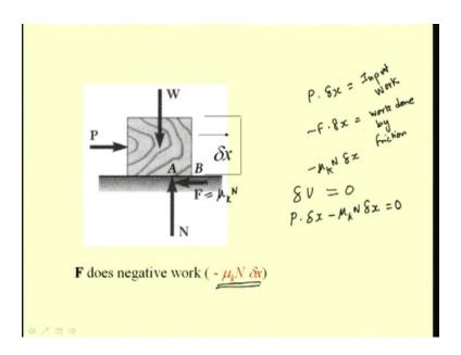
Let us consider the block with friction sliding on a surface which we have used to analyze the problems of friction. Here, we see a block with weight W. A force P is being applied to move this block against the surface. The contact has friction and that is mentioned by this force F. This is the normal reaction N to support this weight.
