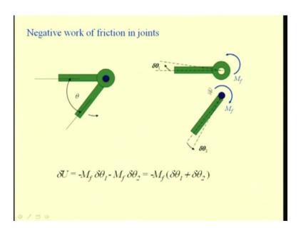
With this understanding, let us try to see how friction acts in the joints of connected rigid bodies. Here, you have these links, two links, connected at this joint.
