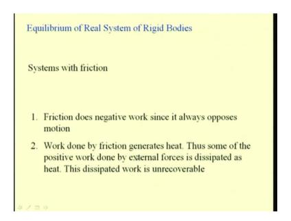
The real systems of rigid bodies are systems with friction. Here, we consider the effect of the friction when analyzing for equilibrium by this method of virtual work. Friction does negative work since it always opposes motion irrespective of the direction of the motion. We have seen that irrespective of the nature of the motion the friction always tends to oppose the motion. Thus,
