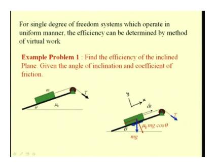
For single degree of freedom system, in these discussions we will limit our analysis of the single degree of freedom systems that operate in a uniform manner. The efficiency can be determined by this method of virtual work.
