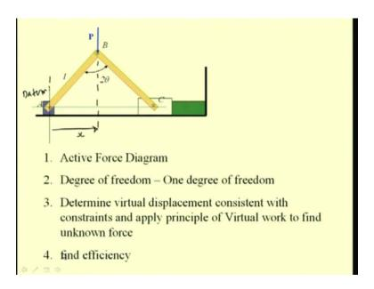
First, let us construct what is called as the active force diagram where we will consider all the forces that will do the work when a virtual displacement is given. So you have to remember that is case of real systems, you have to also consider the frictional forces that exist in the active force diagram because these frictional forces cause a negative work. Then obviously, we have to
