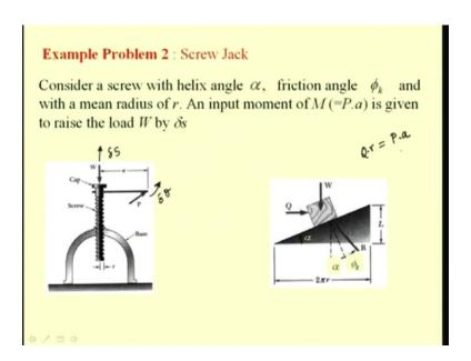
Let us consider another example where the working principle of this screw jack depends upon the friction that is available between the square threads and the base. We have already solved problems of on this screw jack but here we are interested to find the efficiency of this screw jack in raising this load.
