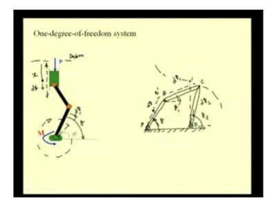
So, we call this as a single degree of freedom system, where we just need one coordinate to specify the configuration completely. So, we can see an another example, like the piston and the connecting rod and the crank, that you normally see in any IC engines; so, this piston traverses a reciprocating motion length, then this crank undergoes rotation. So, the coordinate of this piston say with respect to some datum, say I call it as x can be defined, if I can define this angle theta.
