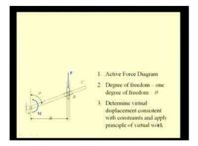
So, let us try to solve this problem by the method of virtual work; so, what will be our strategy? We will first create the active force diagram; here, in this case, we have these two forces, that is P and the applied moment members which do work, for any consist virtual displacement consistent with the constrains.
