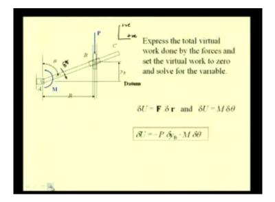
Now, let us express the total virtual work done by these forces and set this virtual work to 0; so, what is the virtual work, that is delta U equal to 0, we have this F dot delta r and the work done by the moment delta U is M delta theta; this work is positive, if both the momentum as well as delta theta are in the same sense and this is negative, if they are in the opposite sense.
