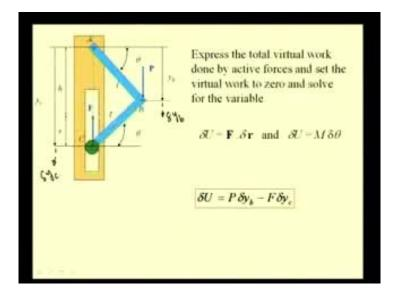
So, now, we can express the total virtual work done by these active forces, that is, this force F and P and set this virtual work to 0. So, we have the virtual work as delta U is F dot delta r and the work done by the moment as delta M delta theta and here, we do not have any active moments; so, this virtual work term is not involved and only we have the virtual work done by the forces.
