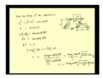
So, this expression now gives the value of the force that has to be supplied by the hydraulic cylinder at this joint, in order to support this weight at this height. So, we see that the method can be conveniently applied to such systems, where it is difficult or not possible to provide detailed information about say the location of this body etcetera and with certain minimal information, it is possible to go ahead with solving for the equilibrium or solving for the unknown forces.
