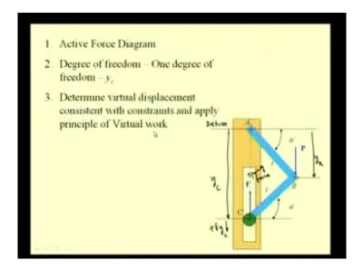
So, what will be our strategy? We will first construct the active force diagram, and then, we will find the degree of freedom of this system; this is a 1 degree of freedom system, because the position of these links can be specified uniquely, if we specify the y coordinate of this point c; so, if we take this as our datum and this as the positive delta y c the direction of the positive virtual displacement.
