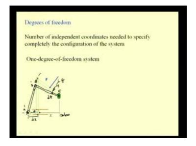
Now, let us define what we mean by the degrees of freedom of a system; the degree of freedom is nothing but the number of independent coordinates needed to specify the configuration of a system completely.
