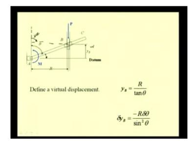
Now, let us define the degrees of freedom of this system, it is a single degree of freedom system, that means, if we define this configuration by this angle theta, then the position of this point B, where the other force P is being applied is uniquely defined. As this angle
