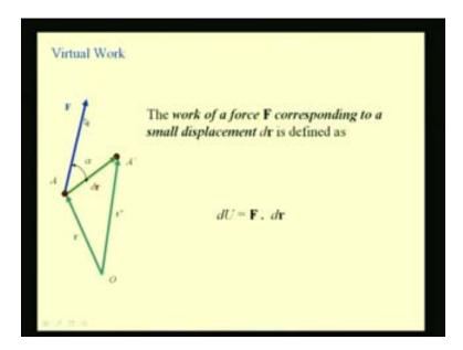
Here, you see a force F acting on a particle A whose position is defined with respect to an origin O by this position vector r. After a small interval of time dt the position of this particle A moves to a new position A prime and the new position vector is r prime and the vector dr gives the
