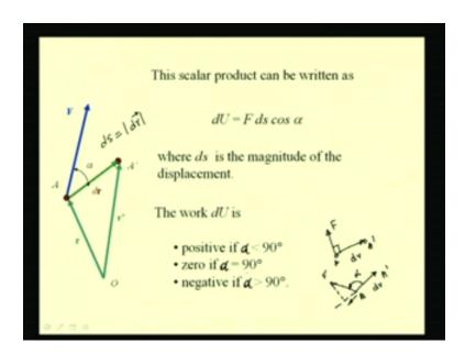
In scalar form, we have dU as Fds where ds is nothing but the magnitude of this vector dr. We define this work dU as F the magnitude of the force vector times ds the magnitude of the displacement vector times cos alpha the cosine of the angle between the two vectors F and dr. This comes from our definition of the dot product.
