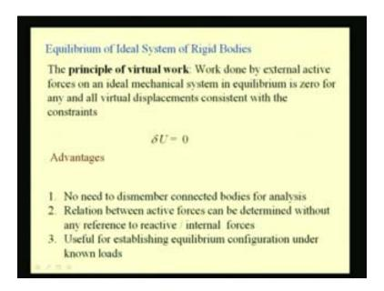
When we apply this equation to the ideal system of rigid bodies, the principle of virtual work becomes the work done by the external active forces on this ideal mechanical system in equilibrium is 0 for any and all virtual displacement consistent with the constraints. We can write this delta U equal to 0. So, the advantage is that we do not need to dismember because we have already seen that the internal forces constitute no work. So, for the analysis we do not need to dismember.
