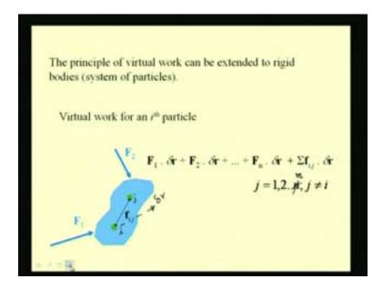
Let us extend this discussion for a system of particles or two rigid bodies. A rigid body is a system of particle where the relative distance between two particles does not change under the action of the forces. Here you see a system of particle or a rigid body and here we are just
