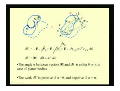
Let us try to derive this quantity based on our understanding that any rigid body motion can be decomposed into a translation and a rotation. Because of the application of this moment M the body has moved from this position to this dotted position. This total moment can be decomposed into a translation and a rotation. Let us take two points on the body A and B and the final position that means on this dotted position we have the positions as B prime and A double prime.
