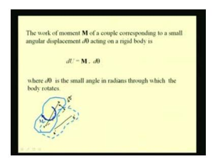
Let us see the work done by a moment. We have seen the work done by a force. So let us see the work done by a moment. The effect of the force is to displace the particle or linearly translate it.
