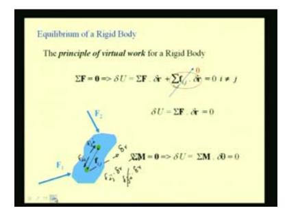
Let us define the equilibrium of the rigid body based on the virtual work that we have defined for a single particle. For this rigid body to be in equilibrium the sum of all the virtual work done by all these forces has to be 0. Let us write that equation. We have this equation sigma F is equal to 0 coming from our equilibrium definition. That means for any consistent virtual displacement the virtual work has to be 0. Let us write this virtual work delta U and equate it to 0.
