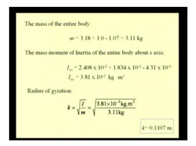
Now, we have determined the second moment of the various components with respect to the x-axis. Now, we can do the required algebra, that is, we sum the second moments of the prism plus the second moment of the semi cylindrical feature and we negate the component corresponding to the hole or the cylindrical feature.
