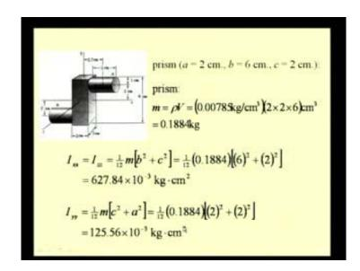
Now, let us move on to determine the second moment of the mass with respect to x y and z-axis for this prism. The various dimensions are that the prism is having a square base; so a is 2 centimeters and c is also 2 centimeters, the length of this prism is the total distance that is we have 3 plus 3 totaling to 6 centimeters; so, the length of this prism is 6 centimeters.
