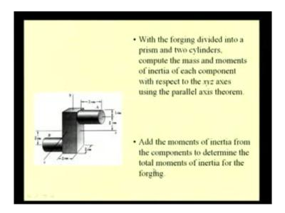
So, what will be our strategy? We will divide the shape into components for which the second moment of the mass is known. So, here we see that this component is made of two cylinders and one prism.
