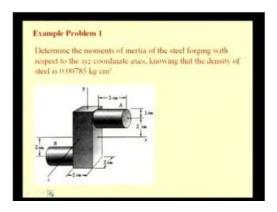
So, let us initially see one example problem to determine the moment of inertia. So, here you see a steel forging and we are interested to determine the moments of inertia of the
