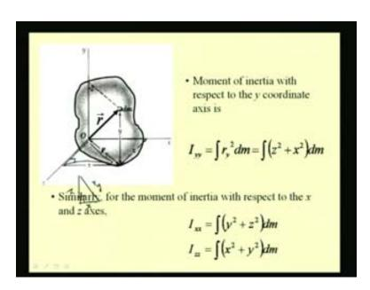
We are interested to know the second moment of a given body with respect to the principal axes with respect to a particular coordinate system. We are interested to find the second moment with respect to x, with respect to y, z, etc., because we have seen earlier that a motion or the angular velocity can be decomposed along their coordinates that is x,y and z.
