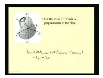
Let us take the perpendicular axis that is CC prime which is perpendicular to the given thin plate. We have already seen how to determine the polar moment of inertia, that means, the second moment of this area with respect to an axis perpendicular to the given plane of the area. Let us now extend the discussion, to the second moment of the mass. Let us say, we are interested to find this second moment of the mass with respect to this axis CC prime.
