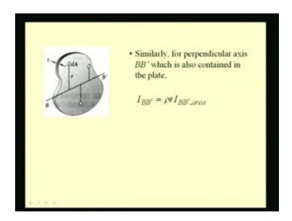
Let us take another perpendicular axis BB prime. Again, we can derive this and prove that this quantity  $I_{BB}$  prime is nothing but the second moment of this plate with respect to this axis. BB prime is equal to rho t which is density times the thickness times  $I_{BB}$  prime area; that means second moment of this area with respect to this axis BB prime.
