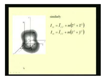
In the same way, we can write for the other two axes that is y prime as well as z prime. We have  $I_{yy}$  equal to I bar y prime y prime plus m, the mass of the body times z bar square plus x bar square. In the same way we have  $I_{zz}$  as I bar z prime z prime plus m times x bar square plus y bar square. In fact, it is possible to write this relation for any axis that passes through a centroid and a parallel axis.
