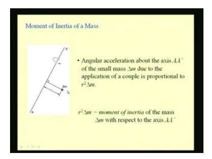
Let us consider one small volume or an elemental volume delta M, which is situated at a distance of r from an axis that is AA prime. The response, that means, if a torque is applied whose vector is along this AA prime will induce a rotation of this mass about this axis AA prime. The
