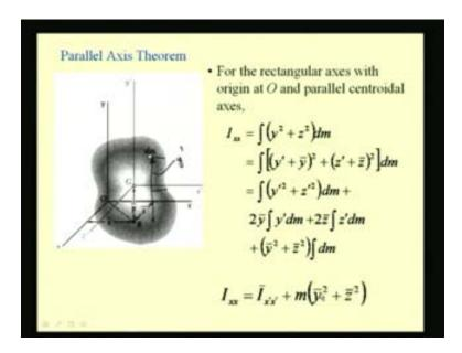
Let us see how we obtain the parallel axis theorem for the moment of inertia of mass. The motivation is again that for a given body if we have obtained the second moments with respect to a given axis, then we do not want to do the same procedure, that is, by the integration in order to find the second moment with respect to an axis system which is parallel. So, we would like to avoid that computation.
