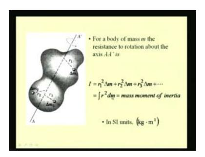
Here, we are seeing one rigid body and we are interested in computing the second moment of this mass or moment of inertia of the mass with respect to this axis AA prime. The moment of this entire mass with respect to this axis is nothing but summation of the second moments of the various particles or various elemental volumes that constitute this rigid body.
