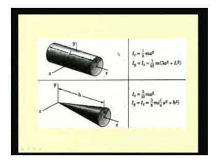
For cylinders, we have, with respect to the axis of the cylinder that is  $I_x$  it is 1 by 2 m a square. In this case, a is the radius of this cylinder and 1 is the length of the cylinder and we have other the two second moments that is  $I_y$  and  $I_z$  as 1 by 12 m 3 a square plus 1 square. Here, you see a cone. Again for the axis  $I_x$  it is 3 by 10 m a square and for the other two axes that is y and z, it is 3 by 5 m times 1 by 4 a square plus h square.
