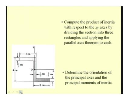
First, we determine the product of inertia with respect to this xy axis by dividing the section into three rectangles. That is, the rectangles corresponding to this area and this area and this area, then we can apply the parallel axis theorem to find the second moments of or the product of inertia of these areas with respect to this axis. Later on, we will determine the orientation of the principal axis and the principal moments. This will be our strategy.
