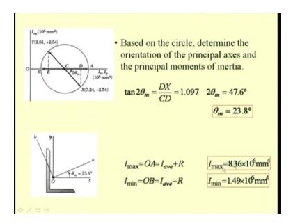
Based on the circle we find that these points A and B, are the points corresponding to the principal moments and the axis has to be rotated by this angle. That is let us designate it as 2 theta m in the counter clockwise direction in order to get the principal moments. So, that means if this is the axis Oxy, then we have to rotate half of this angle in the counter clockwise direction that is theta m, in the counter clockwise direction.
