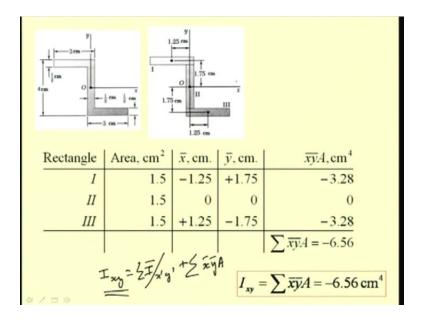
For the area one, we have the area as 1.5 centimeter square, the location of the centroid as minus 1.25 and plus 1.75 and the product of this value that is xy bar A is given here. For this area two, you can see that the location of the centroid is at O, that is 0 and that product becomes 0. The sum of this is minus 6.56.
