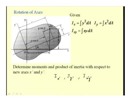
Let us discuss what happens to this product of inertias when the axis rotates. As we developed the theorem for the parallel axis, now we are interested to determine the relation between the product of inertia for two axes which are rotated with respect to a point. We will see that this product of inertia is useful when we determine this relation between the rotated axis and the original axis, for finding the second moment.
