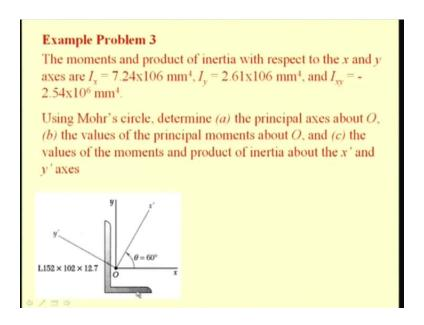
Let us take one typical engineering section, that is an L section and a given axis that is Oyx, about which the values of  $I_x$   $I_y$  and  $I_{xy}$  are known. So, in engineering convention, we represent this section by this notation that is L 152 by 108 by 12.7, which tells the thickness, the width and length of this section.
