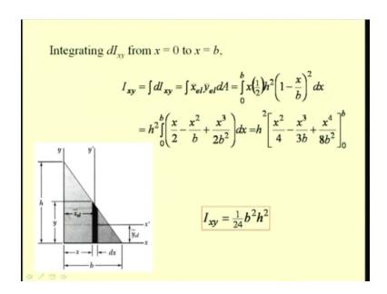
Now we can write the product of inertia of this thin strip with respect to the xy axis as  $dI_{xy}$ ; then we integrate it between the limits that are 0 to b from this to this point. We have  $I_x$  as integral dIxy, which is equal to integral x bar element, y bar element times dA, x bar element is x itself, y bar element is y by 2, which is half of h square into 1 minus x by b square dx into this area.
