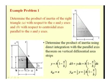
Let us take one example. Here, you see a triangular lamina for which we are interested to determine the product of inertia. It is of height h and base b. We are interested to find the product of inertia with respect to the xy-axis and with respect to the centroidal axis parallel to this xy-axis.
