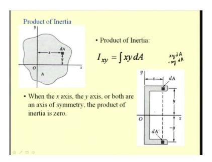
First, we define this product of inertia as for a given area we consider this small element dA, which is situated at a distance of x and y from the axes, x as well as y. We know that the second moment of this area dA with respect to the x axis is nothing but y square dA and the same way the second moment of this area with respect to y axis is x square dA.
