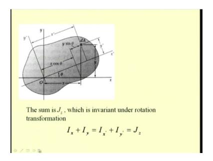
We know that the product of inertia is the product of inertia of the z axis that is the polar axis is invariant when we rotate the object or the axis, that is, the sum of the second moments that is  $I_x$  plus  $I_y$  is equal to  $I_x$  prime plus  $I_y$  prime, which is equal to the polar moment of inertia or the moment of inertia with respect to the z axis.
