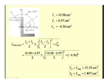
We can also determine the corresponding moments, that is the principal moments, from this equation that  $I_{max}$  comma  $I_{min}$  is equal to I average, which is  $I_x$  plus  $I_y$  by 2 plus or minus the radius of that circle that is  $I_x$  minus  $I_y$  by 2 square plus  $I_{xy}$  square. Knowing these values, we find that  $I_{max}$  and  $I_{min}$  are 15.45 centimeter to the power of 4 and 1.897 centimeter to the power of 4.
