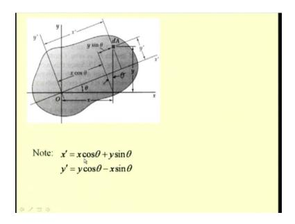
Let us try to relate the coordinate of this area dA in this reference frame that is Oyx and the reference frame y prime Ox prime. In the reference frame y prime Ox prime the location of this area dA is x prime from the Oy prime axis. This quantity x prime is nothing but x cos theta plus y sin theta. We find that this distance is nothing but x times cos theta and this distance is nothing but y sin theta because we have this as y and this angle is again theta.
