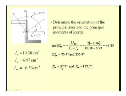
We can move on to find out the principal moments. We know this  $I_x$ ,  $I_y$  and just now we determined this  $I_{xy}$  as minus 6.56 centimeter to the power of 4. We can determine the orientation of the principal axis and the principal moments of inertia. By considering this equation, that is tan 2 theta m, where this angle theta m is the angle of the principal axes.
