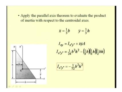
We know the location of the centroid of this triangle and now we want to determine the product of inertia with respect to an axis x double prime y double prime passing through the centroid C.
