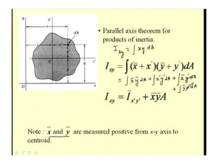
Let us see how to apply the parallel axis theorem for the product of inertia. Here, we have determined the product of this area with respect to an axis Oxy and then we are interested to find the product of inertia with respect to a centroidal axis. So C being the centroid of this area, we have the parallel axes, that is x prime y prime, passing through the centroid.
