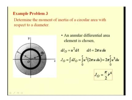
Let us take one example. Here, we see a circular area and we are interested to find the moment of inertia of this circular area, with respect to this diametrical line, say, with respect to this x-axis.
