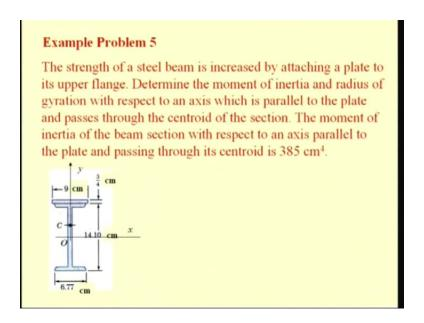
Let us see one example, here you see a typical I section, cross section for a beam. In order to strengthen this, we are actually welding a thin strip or a plate to the top of this I section beam. We are interested to find the moment of inertia and the radius of gyration, with respect to an axis which is parallel to this plate and which passes through the centroid of this section.
