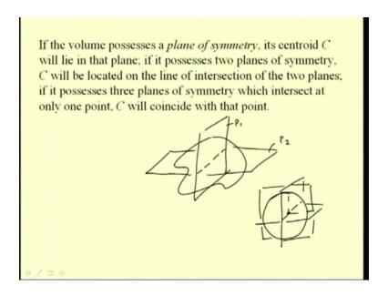
We have seen in 2D, that, if we have a line of symmetry for a plate, then, the centroid lies along that line of symmetry. Because, the moments, the first moment of the differential elements are
