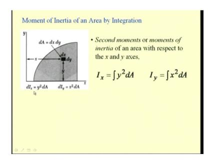
We can determine the moments of inertia of an area with respect to x and y-axis. We define it has  $I_x$ , the second moment of the area as integral y square dA. If we take this picture, we are interested to find the second moment of this total area. We take a small differential element dx dy, which is situated at a distance of x from the y-axis and at the distance of y from the x-axis.
