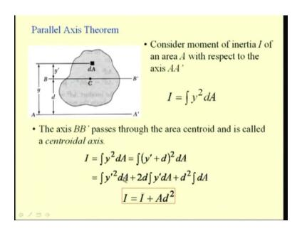
If we determine the second moment with respect to a given coordinate system then we can determine the second moment with respect to a parallel axis. Because, if in a particular engineering calculation, the area is now transformed with respect to a given axis, its second moment changes, but we are not interested to compute every time the second moment by let us say a method of integration.
