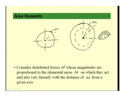
So, let us consider a solid sphere, which is having the centroid at its center and another sphere which is hollow from inside; that means, when you will cut it, you will have something like this. The inside is hollow for this solid. Also, we will see that the centroid lies in the same location. If
