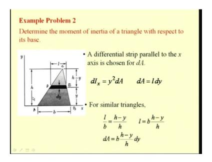
Let us take this example problem. Here, you see a triangle for which we are interested to find the second moment of this area with respect to its base; that is in this case, with respect to the x-axis because the base is located on the x-axis. In order to do that, we define a thin horizontal strip of width dy, which is located at a distance of y, from the x-axis.
