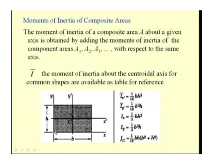
If we have composite areas, then we can determine the second moments by considering the second moments of the individual areas and summing up in order to determine the second moment for the component or the compound area. For simpler shapes these are known. For this rectangular area we have these various quantities like the second moment with respect to the centroidal axis, say x x prime or the centroidal axis y prime and the polar moment of inertia of
