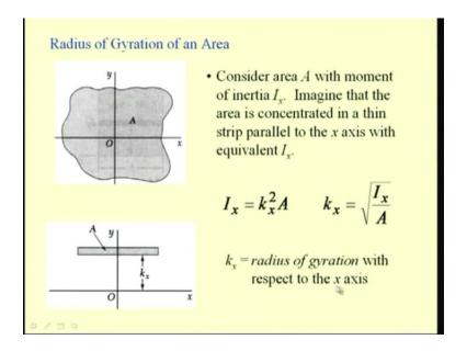
We define this radius of gyration of the area. For defining this for any element or any area element, if we assume that, this element is of a form of a thin strip and if we want to equate the second moment of this thin strip to the second moment of the area then the distance at which this thin strip will be situated is known as the radius of gyration.
