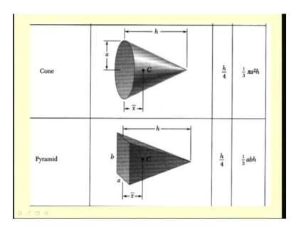
In the same way for other simple solids, like cone and pyramid, the location of the centroids can be found. In case of cone, again we have symmetry. It lies along this axis and lies at a distance of h/4 from the face of the cone. For this pyramid, we have the centroid located at h/4 from this base.
