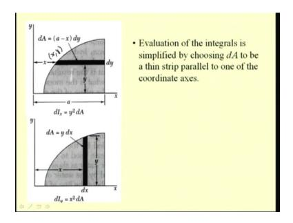
Here for the same example, we take a thin strip which is horizontal or parallel to the x-axis. In order to determine the second moment of this area, with respect to this axis, that is x-axis, we define the second moment of this thin strip  $dI_x$ , with respect to this x-axis as y square, the distance square from the axis times dA, the area of this element.
