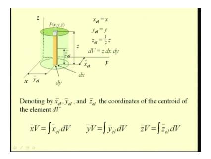
We can find these locations of the centroid x bar, y bar and z bar by this integrals; that is x bar V, where V is the volume of this cylinder is equal to integral x element bar dV, and same way, for the location of y and z coordinates of the centroids can be found.
