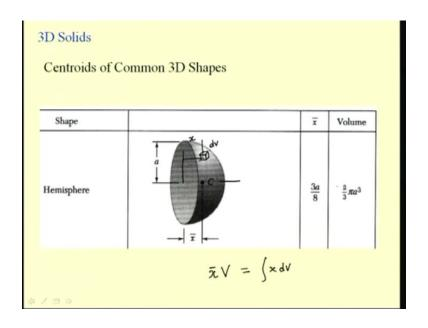
For 3D solids, the centroid can be determined by the integration and for common shapes these values are known. Again, for 3D solids, we determine the centroids by finding the first moment of the differential weights of the small elements that we take and then, we integrate it to find the location of the centroid.
