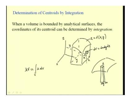
Centroids can be found by the method of direct integration for analytical surfaces. If we take a surface whose equation is of the form, Z equal to function of x,y; the surface is an analytical surface. Since we have the definition of the surface in terms of these coordinates, we find the centroid of the volume under this surface, by considering a small element whose volume is dv, which is equal to dx dy dz and which is located at distances, say y, z and x.
