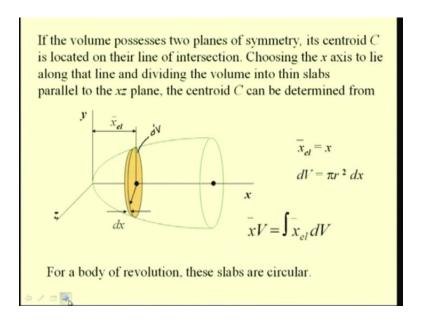
Here, you see an example, where we have two planes of symmetry, that is, this object is symmetrical about this plane yx, as well as it is symmetrical about this plane zx. The centroid lies along the line of intersection of these two planes, that is, the x-axis. We are interested to find the location of the centroid, along this x-axis. For that, we consider this thin slab which is
