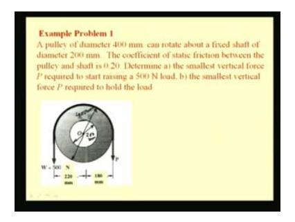
Let us take one example problem and see how we solve the problem of this journal bearings. Here you see a pulley supported on a shaft at O. The diameter of the pulley is given as 400 mm and it can rotate about the fixed axis shaft of diameter 200 mm. This axle or the shaft is having a diameter of 200 mm; this is 200 mm and this has been given; as this is the radius, we have it as 200 mm and the diameter of the pulley is given as 400 mm.
