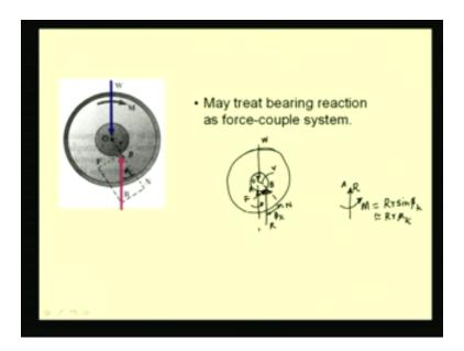
We can treat this bearing reaction R at this point B as a force and a couple system. Let us see how to do that. We have this wheel and the axle, the weight passing through O and the point of contact has shifted to this point B. This is the normal reaction and we have the frictional force and the resultant R. This is small r the radius of the axle.
