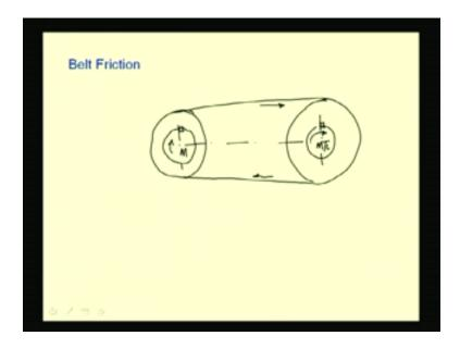
Let us see another application of friction that is employed in belts for transmitting power from one shaft to another. Let us consider two shafts, one which is connected to the motor and the other to a rotating machinery. The torque that is developed by this motor has to be transmitted to this machinery. This can be done by many ways.
