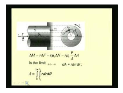
Let us consider a hollow shaft as shown in this picture. Let  $R_2$  be the outside diameter and  $R_1$  the inside diameter of this hollow shaft which bears onto this support in this N
