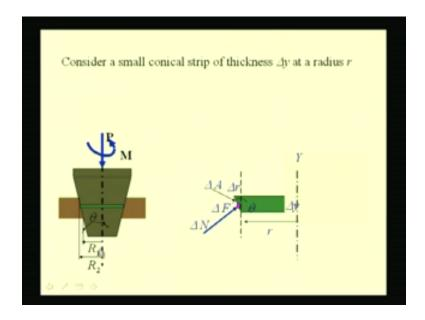
Let us say this axis is y. Then, we consider this differential element, which is a thin slice of this conical pivot bearing. Let us draw the free body diagram of this element. Here, this vector which is perpendicular to the plane of the paper is the frictional force delta F corresponding to this area; delta N is the normal force and since this moment M is in the clockwise or the counter clockwise direction to this force, del F is moving inside the plane of paper or this plane of the board.
