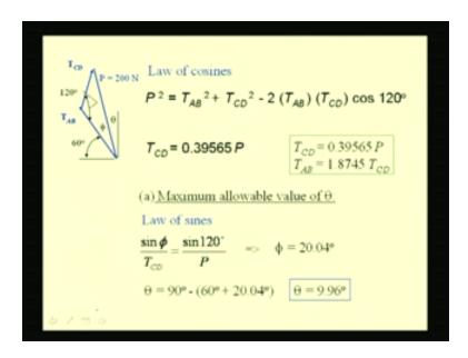
Let us consider this force triangle, where we have marked these forces; that is  $T_{CD}$ ,  $T_{AB}$  and this 200 Newton force by these vectors. So we have this 200 Newton force which is having an angle of inclination of theta, with the vertical, the force in this cable CD and the force in the cable AB. The angle of inclination of these two vectors is known from the geometry.
