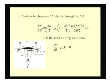
Let us eliminate this delta N from these equations by dividing it throughout by delta theta. So we get delta T by delta theta cos delta theta by 2 minus  $mu_s$  times T plus delta T by 2 times sin delta theta by 2 divided by delta theta by 2 equal to 0. If in the limit, that is delta theta tends to 0, this equation becomes dT by d theta minus  $mu_s$  times T equal to 0, because this quantity, the product that is delta T times sin delta theta by 2 is negligible and this becomes 0.
