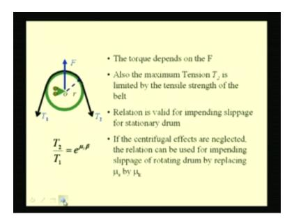
We see that the torque depends on F and also depends on this maximum tension  $T_2$ , which is limited by the tensile strength of the belt. This relation we have found for the impending slippage for stationary drum. If we discard the centrifugal effects, then this relation can be extended to impeding slippage in the running condition by replacing the coefficient of static friction by the coefficient of kinetic friction.
