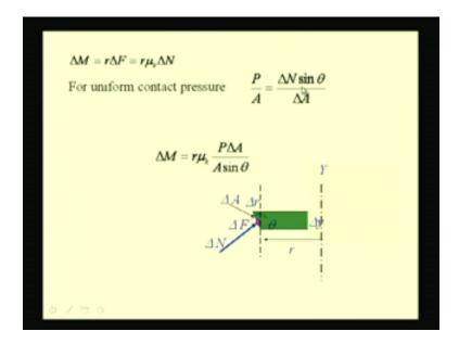
So, the frictional moment that has to be resisted for this differential element is delta M, which is equal to r times, which is the momentum, the frictional force that is delta F. For the constant motion case, this frictional force delta F can be related to this delta N by the coefficient of kinetic friction  $mu_k$ . We have delta F equal to  $mu_k$  times delta N. So delta M is  $r mu_k$  delta N.
