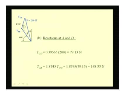
Now, we can determine these two tensions  $T_{CD}$  and  $T_{AB}$ , which are nothing but the reactions at A and D. They are 79.13 Newton and 148.33 Newtons. So this example illustrates solving problems on belts and finding the required friction or the tendency of slippage between the belt and pulleys.
