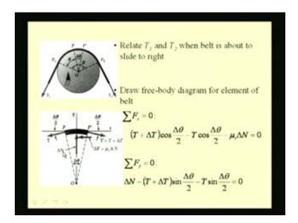
Because, the motor drives this pulley, the tension that is developed is larger on this side, which is depicted on this picture. Let us say this is the pulley. We have the belt element passing over the pulley and the tensions on the two sides being  $T_1$  and  $T_2$ . Let us also assume that the belt tends to slip to the right hand side. That means the tension  $T_2$  is larger than this tension  $T_1$  and which is pulling and trying to rotate this pulley about this point O.
