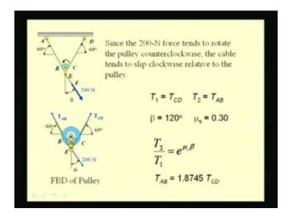
Let us proceed by considering this diagram, where we have this force of 200 Newtons that is being applied at an angle of theta. We are interested to know this angle for the equilibrium position. This 200 Newton force tends to rotate this pulley in the counter clockwise direction. So, this force tends to rotate this pulley in the counter clockwise direction. Since the cable that is fixed at A, passes over the pulley and goes to D, the cable tends to slip clockwise relative to the pulley.
