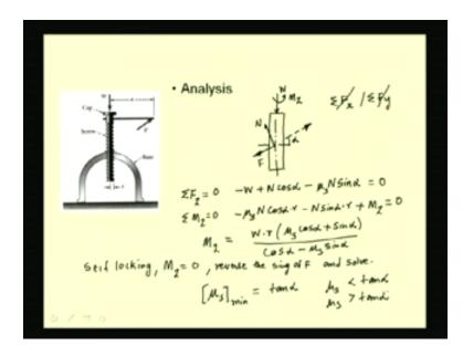
Let us consider that free body diagram. Let this be the screw. We have the weight and the applied moment, M<sub>z.</sub> This is the sum total frictional force acting on the thread face and this is the sum total normal force acting on the thread face. This free body diagram is an equivalent free
