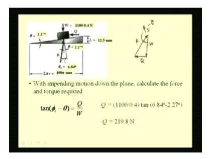
Once we have created this equivalent diagram, we can write the force equation.
