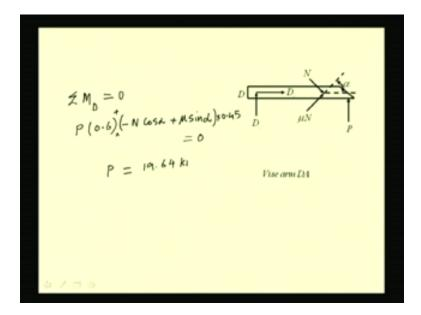
Let us move to the next free body diagram that is the y sum. This shows the free body diagram. Here, we have already computed N and we can compute force P, if we take a moment equation about this point D. Let us write that equation.
