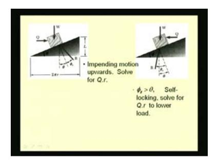
If we have the impending motion upward, it is equivalent to raising the load by applying the required moment on the screw jack. This is the equivalent free body diagram of the inclined plane. The reaction force which is the sum total of the normal reaction and the frictional force on this face, makes an angle of phi<sub>s</sub> with respect to this normal. If theta is the lead angle then the normal of this inclined face, makes an angle of theta with this vertical.
