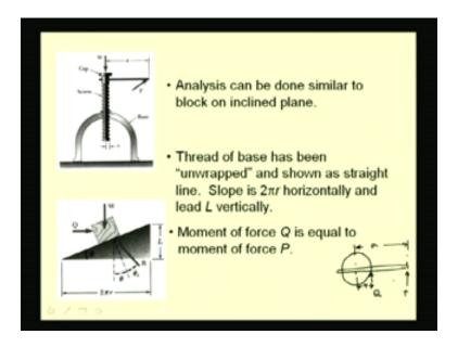
The analysis of the screws that we have seen can be done by another method, where we analogize the problem to that of a rising the load on an inclined plane. Let us consider this screw jack again, where we apply force P to cause a moment to raise the load W. We draw an equivalent inclined plane, by unwrapping the thread on the plane of paper. We know that if we rotate the screw by one revolution then this load W, is raised by a distance equal to the lead of this thread.
