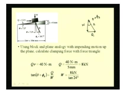
Let us construct an analogical inclined plane. This plane has a lead of 4 mm. This is the lead angle which we have found as 7.3 and this is the angle of friction phi<sub>s</sub> which we have found as 16.7 degrees. When we apply the moment, it is represented by an equivalent force Q on this inclined plane which is used to raise this weight. In this case, this W is the force that is being applied on the blocks.
