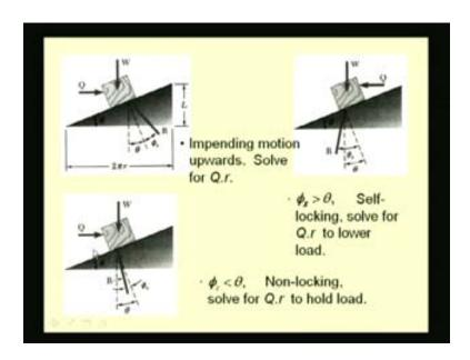
This diagram represents, for the impending motion upward, where the force Q pushes the weight against the slope. If the thread is a self-locking thread then if we leave the load on the inclined plane, it will not slide down. So, that is the equivalence to a self locking thread; that means, we need to apply a force Q in order to push this load down the inclined. We can consider this free body diagram and find the required force Q; Thus, in turn, the required moment in order to lower the load.
