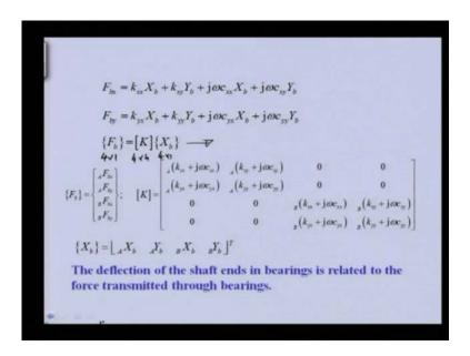
So, if you go back to the previous here we related the bearing force with the bearing displacement. So, this relation we can able to use here.
