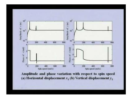
So, you can able to see this is the response in x direction and the phase of that. So, there are 2 critical speeds we can able to see in this because linear motions. So, here we have getting 2 critical speed third is also there these not seen here, but in y direction where we can able to see the third critically speed also, and there is phase change where there is these critical speeds are there here also, three critical speed. The fourth one was not visible for values we are chosen.
