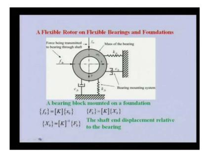
In the previous figure we have seen that the bearing mass is having in x and y direction.
