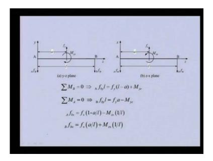
So, you can able to see this is the free body diagram of the shaft, we removed the disk from the shaft. So, the reaction forces M y and moment M y z from the disk on to the shaft is acting in the, positive in these directions, because these are reactions. So, they will acting in the positive y and positive displacement, angular displacement direction. Now because of this the 2 end of the shaft A and B were removed from the bearing also this particular shaft.
