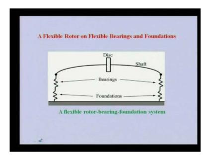
So, here you can able to see that we have disc, shaft is flexible bearing is there and then the pedestal or foundation is there. So, we have basically we need to obtain the effective stiffness, how this particular disc is experiencing at the bottom of due to the shaft bearing and foundation.
