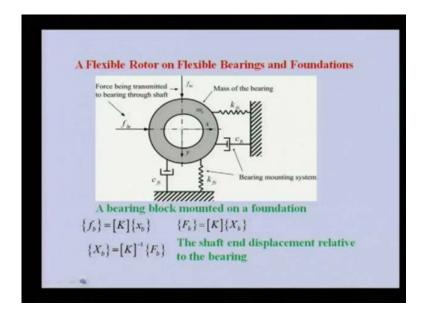
So, I am coming to the free body diagram of the let us see the bearing. So, this is the bearing mass in the previous analysis we did not consider the bearing mass now, this is the bearing and general we have removed from the bearing. So, obviously, the fluid fill forces which is coming what are the bearing mass is f b x in x direction f b y in the y direction these are the fluid fill forces which are coming on to the bearing mass.
