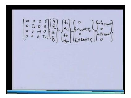
So, this particular four equation, we can able to write like this. So, this is the equation of motion, this is the mass matrix which will be coming from the inertia term of the four equations. So, you can able to see that we have arranged the various variables like y
