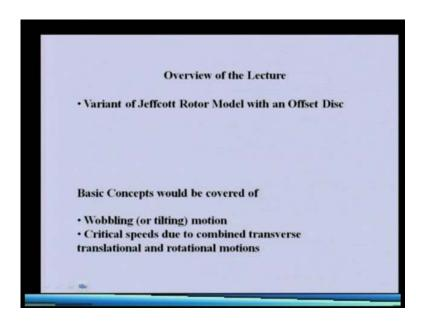
This is the overview of the lecture in which, we will be taking the variant of the Jeffcott rotor model, in which the disk will be offset some of the concept, which we will be seeing is the wobbling motion or the tilting motion of the disk along with the translatory motion and then we will be studying the critical speed due to the combined transverse and rotational motion of the disk. So, in this particular case let us consider.
