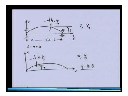
A flexible shaft which is supported at ends with friction less bearing let us say this is simply supported at ends. And there, is a disk which is offset from the centre this is the disk, this is the bearing axis. So, let us say this is z axis let us say vertical axis is y, and there is another axis which is perpendicular to the plane of screw, we will consider that subsequently let us say we are considering the motion in this two plane at present.
