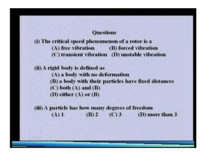
The critical speed phenomena of a rotor is a as we know the critical speed is the speed at which, the natural frequency is equal to the spin speed and in this particular case speed of the rotor is important and this particular phenomena is gone by the unbalance force and because of this critical speed concept, which is a resonance phenomena is a force vibration phenomena, this is not a free vibration even not a transient vibration or unstable vibration.
