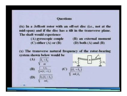
Now coming to the next question, we have already seen a jeffcott rotor with an off-set disk. So, if it is not at mid span obviously, we have seen that the tilting of the disk take place in the transverse plane and this would not only additional external moment, but also it will give a gyroscopic couple, which will be seeing in subsequent lectures, that this particular disk is spinning and is having precision about it is diameter. So, gyroscopic couple would also be acting.
