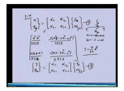
So, I am writing those two equations in a one matrix form. So, this will combine the 2 equation in 1. So, if I simply supported beam generally, this influence coefficient matrix take the following form just for illustration, I am giving the if, let us say we have simply supported beam these are the support.
