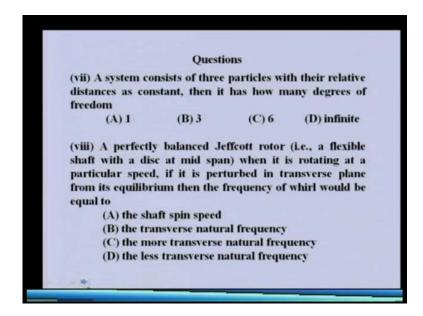
Now if we have a system consist of three particles we already seen that three particle, if they are having no relative motion that represent a rigid body. So, three particle with their relative distances constant then it has how many degree of freedom so obviously, a rigid body we are referring to and it has 6 degree of freedom system, now a perfectly balanced Jeffcott rotor.
