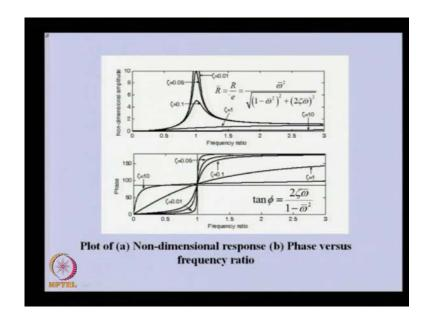
You can able to see the horizontal axis is the frequency ratio of the first plot and non dimensional amplitude, complex amplitude is in the second and you can able to see it has been plotted for various damping. At zero damping it will be at very high amplitude will occur and the frequency ratio 1, but as the damping increases this peak across that will less than this frequency ratio, because this frequency ratio has been defined with respect to the undamped natural frequency.
