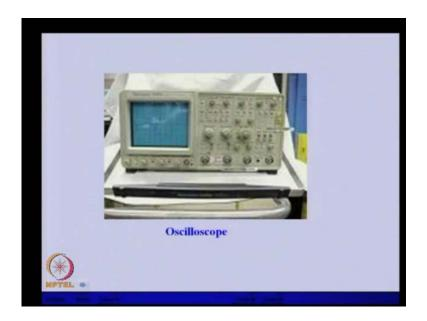
This is for displaying the whatever the vibration signal captured through this these sensors. We can able to display the signal on this kind of screen that is the oscilloscope. Generally, it is it displays signal in time domain. But, frequency domain signal also can be seen in this.
