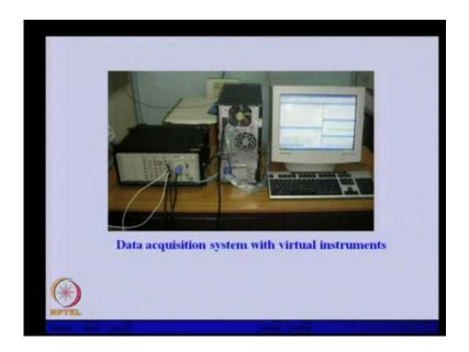
Various form of the signal in the frequency domain can be plotted apart from the FFT simple FFT. Or if required, we can able to transfer the data into the computer through a data acquisition system, and here we can have some kind of virtual instrument. So, depending upon the need what kind of processing we want to do, we can able to make our own instrument virtually.
