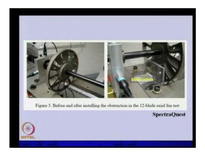
So, before and after installation the observation in the 12 blade axial fan so there are 12 blade axial fan, in this we put this is taken form a spectra quest lecture nodes. So, this is the obstruction, which was put here so that, we can get some kind of disturbance.
