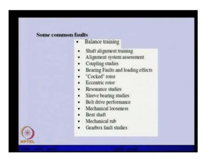
So, these are the various kind of faults generally as we have discussed in the previous lecture also various kind of faults. We can have, and every fault gives a unique frequency in the vibration spectrum and with the help of that unit frequency, we can able to identify which kind of fault has appeared in a particular machine.
