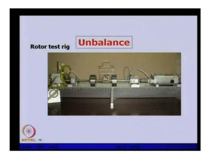
Now, coming to the unbalance, we already seen how the procedure how to balance a rotor. So, it is a typical rotor in which this is a motor the bearings are there here. It is a
