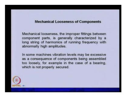
The improper fitting between component parts is, generally characterized by a long string of harmonics of running frequency with abnormally high amplitudes. In some machines vibration levels may be excessive as a consequence of component being assembled too loosely. For example, in the case of bearing, this is not properly secured.
