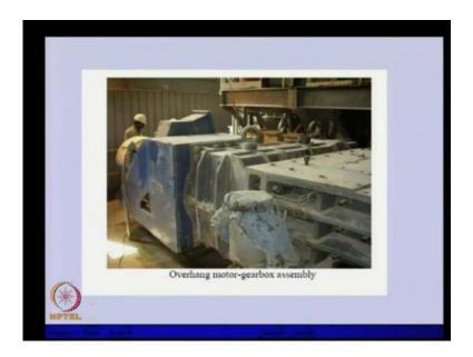
So, in this is a typical industrial stone crusher. Basically, here motor is there. Drive is there. Then, this is the coupling unit, which we can able to see it. We have then this side. There was one crusher unit, in which the stones used to crush from bigger to smaller size. In this particular case they had lot of problem of the vibration. Basically this whole unit was mounted on a plate form. If we...So, basically it was in the first floor kind of thing.
