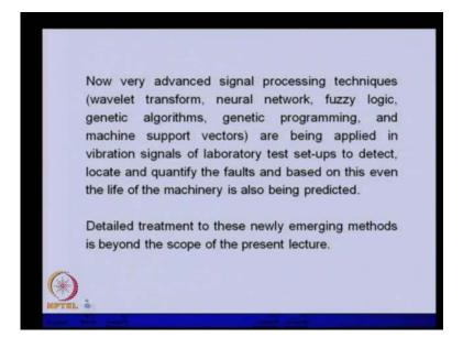
Now, very advanced signal processing techniques like; wavelet transform, neural network, fuzzy logic, genetic algorithm, genetic programming and machine support vector SVM, are being applied in vibration signals of laboratory test setup to detect, locate and quantify the faults. Not only the detection of the fault, now with these techniques we can able to pin point, where is the fault and even we can able to quantify the fault.
