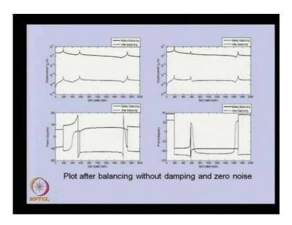
Now, when we are comparing the responses, this is without a correction mass and this is without balancing. So, this is after balancing. So, whatever this estimated correction mass we calculated, we kept into the balancing plane. Then we found that the responses are drastically reducing in both the plane. Here, also you can be able to see the response drastically reducing.
