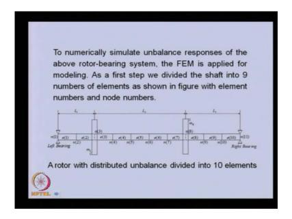
So, this is the rotor. So, we divided this into 10 elements and various nodes and the elements are mentioned here. All geometry of the rotor we know. So, we can be able to obtain the elemental equation for a rotor.
