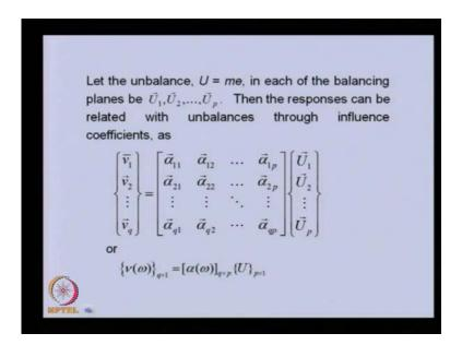
So, in this we have this is unbalance as we defined earlier which is nothing, but mass into eccentricity. In these planes, the balancing planes let us say U 1, U 2, U p, these are the unbalance which we want to find out. These are the corrective unbalances, which we need to find out. Now, these are the equivalent unbalances corresponding to the
