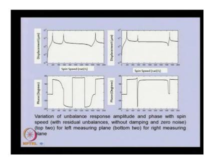
So, this is the typical plot of the unbalanced response in which we have shown this is the amplitude versus speed and this is the phase verses speed. In this, we changed the speed of the rotor beyond the third critical speed, so this is the third critical speed, first, second and third and in the phase plot you can be able to see there is a change in the phase wherever there is a change in the phase. Here also, these changes are basically because the phase is cyclic.
