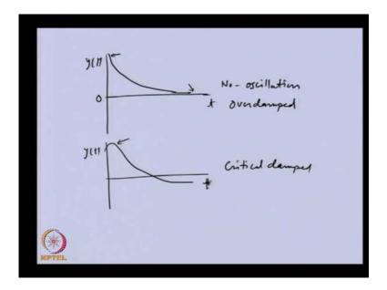
Here you can able to see when over damped system is there, we or let us cut this one. For over damped system we will be having a response like this. There will not be any crossing of the response from the 0 line. So, after sometime gradually if we are giving some disturbance to the system from here resonate will come to the rest. It will not cross, there will not be any no oscillation will take place. This is for over damped system.
