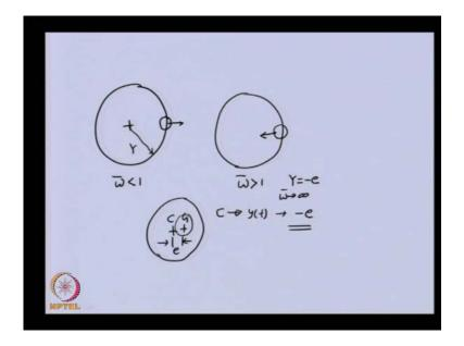
So, earlier we have seen that the volume of the shaft about its varying axis and when we are operating below the critical speed, that is frequency ratio 1. The unbalance force is towards the outward direction and this is the amplitude Y which we are talking about in the previous analysis. But the same thing when we were cross the critical sped, this particular unbalance force comes towards the negative direction. We have seen that the Y becomes negative at very high value of this.
