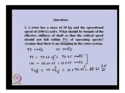
Can I take one example? Three minutes I can take one example, I will speed over the three minutes. So, let us take one question. A rotor has a mass of 10 kg, the operational speed is 10 plus minus 1 radians per second. What should be bound of effective stiffness of the shaft, so that the critical speed should not fall within 5 percent of operating speed? Assume that there is no damping in the system.
