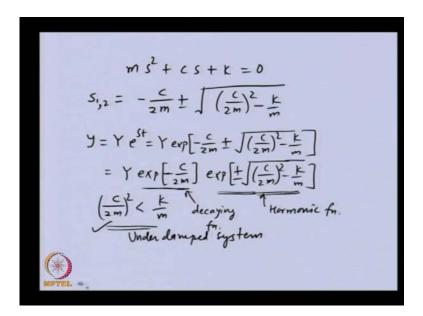
So this is the equation of frequency equation we got form the spring mass damper system. We can able to solve for s because this is a quadratic equation. So, we will get two roots and the solution will be of this form, and if we substitute this in the assumed solution. Let us say I am writing this as exponential and within the bracket these terms. Now, this can be written as we can able to separate it out some of the terms like this. And we can take this square root term separately.
