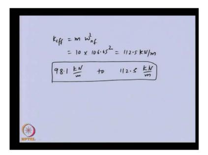
And if we see the upper range, so that is again you can able to substitute this. But in this particular case we will be having the frequency upper limit of the operating speed this much. This will give us 112.5 kilo Newton per meter. So, that means the natural frequency should not fall between range. The previous one is 91, 98.1 radians per second. Again I am repeating this.
