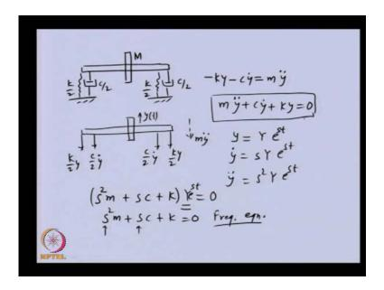
So, in this particular case let us say we are considering a simple rotor system which is rigid shaft and a mass. This is supported on a spring and mass spring and damper system. Let us say the damping is viscous damping and the coefficient is c, stiffness is half, k by half, k by 2. Here c by 2, k by 2. This is M. So, in this particular case you can able to see
