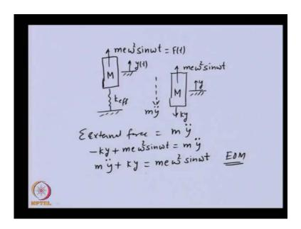
And all these models we can able to represent by a mass and a effective stiffness of the support or of the shaft. Mass is having value M and we are having some kind of displacement in vertical direction which will be time dependent. If you consider the previous model, let us say the first one or second one. We can have some kind of centrifugal force due to the unbalance of the mass and that we can able to apply on this particular mass like m e omega square sin omega t.
