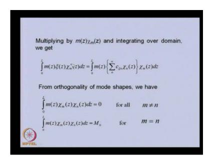
So, Eigen function and also mass per unit length and we are integrating over the domain. So, in previous expression e are multiplied by two terms and we are integrating over the domain. Both sides we have multiplied and here you can able to see. Again we can able to use the orthogonality condition to simplify this. So, whenever these two functions are
