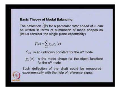
So, this particular case the deflection of the shaft in zai direction which is, which will be in the function of z and when we are talking about the flexible rotor then we need to talk about at what speed we are operating. So, this deformation deflection ((Refer Time:
