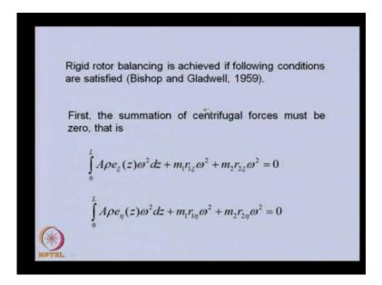
Let us say for rigid case, in this case whatever the summation of centrifugal force are there due to the variation of eccentricity of the rotor itself, this is the eccentricity, this is the mass on unit length. We multiply by z, that will be mass of the rotor of a slice and because this is eccentricity, so that is the total unbalance. If we multiply by omega square that will be the centrifugal force, this we are integrating over the whole length of the shaft.
