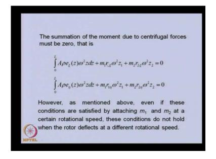
So, this is the total centrifugal force acting in the z i direction due to the rotor eccentricity and these are the correction mass. Correction mass component of the centrifugal force in this A n z i direction. So, this should be balanced, so whatever from the eccentricity rotor and correction masses should balance in this plane, not only in other plane. The eta direction also it should balance the centrifugal force.
