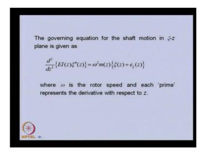
Now, we will take up the governing equation of the shaft in continuous system approach and we have to king this in the zai z plane. So, this is the equation of motion which we derived during the transverse vibration of vibration using continuous system approach. So, you can able to see this prime is basically is the derivative with respect to z to prime is double derivative with respect to z, similar to this derivative.
