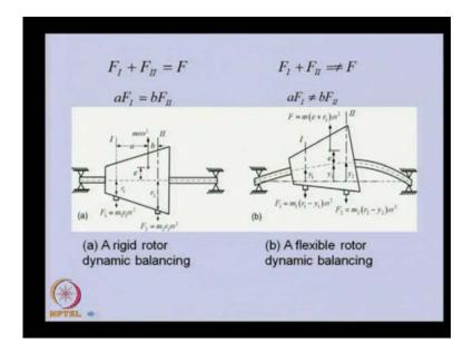
So, with this figure this is the rigid rotor balancing the rotor which we discussed earlier in which we tried to balance the eccentric rotor with two planes. So, for this we plane have F as the unbalance force and F 1 and F 2 we are putting the correction masses. So, centrifugal force these condition we need to satisfy to balance the rigid rotor, not only this one, but also the movement.
