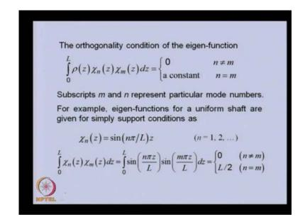
So, this is the autocratically condition in general. So, this we already discuss earlier that if m is not equal to n, then it becomes 0, n is equal to same then it is constant quantity. For simply supported rotor case we have this as the Eigen function. Earlier we obtain this also and we substitute this Eigen function. In this integral we see that when both are not equal, this quantity will be 0 if m is equal to m, this will be L by 2.
