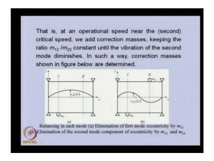
So, basically now this is summary, we balance the first mode by one mass. Then the second mode by two masses, like this you can able to do the second mode and the total balancing is the submission of this two.
