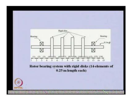
So, in this particular case just to show the convergence we have taken two cases, one is we have idealized this as 7 elements. In this second case we have considered that as 14 elements. So, we have divided this various shaft segment into two so that the number of elements becomes 14.
