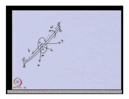
So, I will explain this by simple Jeffcott rotor, so in this we have one Jeffcott rotor like this where this is the ((Refer Time 04:33)) disc? This is mounted on some rigid bearing, may be rolling little bit bearing, so flexibility of the bearing we are not considering. Apart from this we, so here we can able to take, this is the un-deformed, so this is the
