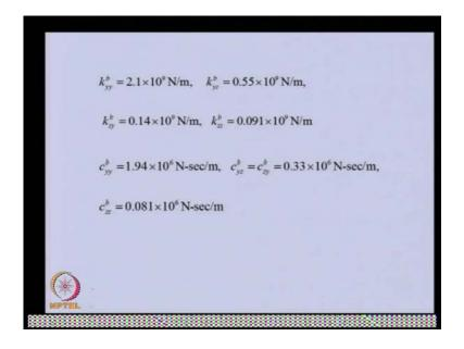
So, these are the by short bearing approximation which we described earlier, for mean speed of 4000 rpm and various bearing property. We can able to bearing parameter, we can able to get the stiffness coefficients and damping coefficients of bearings like this.
