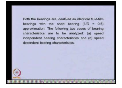
They are idealized as identical fluid film bearing and they are 1 by deviation is 0.5, which we can able to consider as short bearing. We need to consider two cases, one is speed independent bearing characteristics. In this we are considering we are choosing one bearing parameter, we will keep constant that during the change of the speed. In this particular case another is speed dependent bearing characteristics in which we will be varying the speed of the property of the bearing with the speed.
