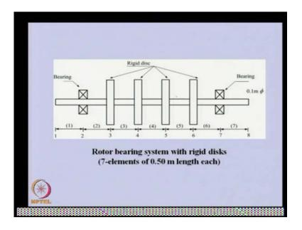
So, in this particular case we are taking basically a rotor system like this, so there is a huge rotor with four discs are there, they are also heavy discs. These bearing fluid film bearings and we will be modeling this particular rotor system using finite element method, various property of the rotor and bearings are given here.
