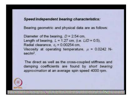
So, for speed independent bearing characteristics various parameter of bearing like d l where algorithm is this radial clearance, viscosity at operating temperature we have provided. So, direct as well as the cross coupled stiffness and damping coefficients, we can able to find for any particular speed. So, what we have done at 4000 rpm, we have obtained the bearing property and we are assuming that remains constant for all other speed, so something like average speed we have chosen.
