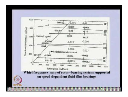
Now, we are calculating the stiffness and damping parameter that is variation of the, they are varying with the speed. So, when we discussed this particular short bearing approximation in previous lectures, so because they were in the non dimensional form. So, in this particular bearing we can able to get those parameter and we know that they vary with speed, so those values we have directly fed into our programs.
