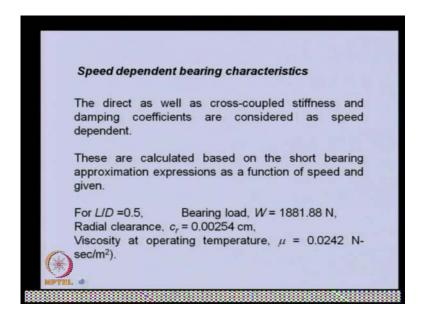
Then next we will be considering the speed dependent bearing characteristics, in this direct as well as the cross coupled stiffness and damping coefficients are considered as speed dependent. These are calculated based on the short bearing approximation expressions as function of speed, so here these are the same bearing parameter.
