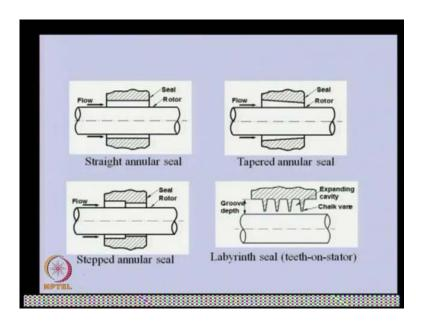
So, in rotors system, we will find various kind of seals like let us say, rotor which is rotating about its own axis. This is the either, this is stator and basically this is seal which is provided generally to stop or to minimize the flow of the working fluid or the lubricant from one end of the shaft to another one. So, here simple surgical shape is there of the seal. Generally, the seals are having larger clearance as compared to bearings.
