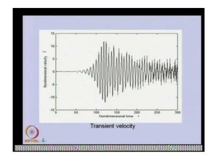
In this particular case, again this behavior is there because there is a angular acceleration of the rotor. This is this is the transient velocity, in place of displacement velocity is there.
