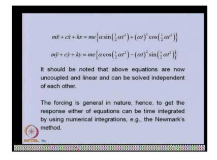
And now, like this, now and so basically, here now we will be obtaining this because here the forcing is general in nature because this is external force. Because of angular acceleration, the force is not a linear. It is varying continuously with time, so we will be using some kind of time integrated integration method, numerical method like Newton new marks method we can able to use it.
