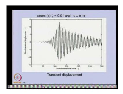
So, this is a typical non dimensional displacement x-prime with non dimensional time. So, you can able to see with time how the response changes. This is for one particular case.
