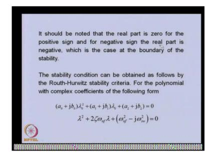
So, one of the root gives the boundary of instability and another is giving the stable solution of this. Now, we should be noted that the real part is 0 for the positive sign and negative sign, the real part is negative which is the case at the boundary of stability, that we are yet to discuss. The stability condition can be obtained as follows by Routh-Hurwitz stability criteria.
