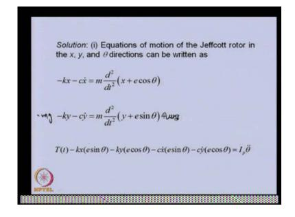
So, you can able to see apart from the stiffness, we can able to add the dumping force also. This external force should be equal to the mass into angular acceleration and this is the angular position, this is the linear position of the center of gravity of the rotor.
