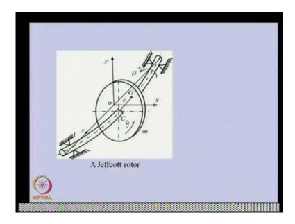
So basically, the rotor is like this; x, y and z is in this direction and is rotating with contact clockwise direction, which is theta direction. This is theta velocity. Now if we take the free body diagram of this, we will see that these are the elastic force from the shaft.
