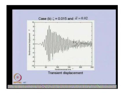
So you can able to see, these is the resonance after that there is a this kind of non-transient behavior. This is for another case, similar plots are there, for different damping and angular acceleration, so these are this for velocity. This for approaching resonance. This is for terminating resonance.
