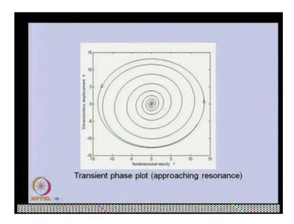
This is the basically the plot of the x and the x dot, x-prime and the x-prime dot. So, this is the phase plot, transient phase plot. So, when resonance is approaching, we can able to see the gradually the amplitudes are increasing.
