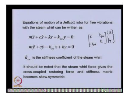
So, let us see the equation of motion, of a Jeffcott rotor and in which the steam whirl is taking place. So, for that, these kind of equation of motion is valid. So, you can able to see the first 3 term is belonging to the rotor, but this is due to the steam whirl. So, basically steam whirl stiffness is coupling the y direction equation of motion with the x
