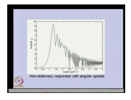
And this is with angular velocity, how the transients are coming once we are going away from the resonance condition. Today, we have seen one is the stem whirl and how the steam whirl can give instability to the system and how we can able get the condition of instability, which are the parameter which can govern the or which can able to stabilize the system, in which there is a possibility of the steam whirl.
