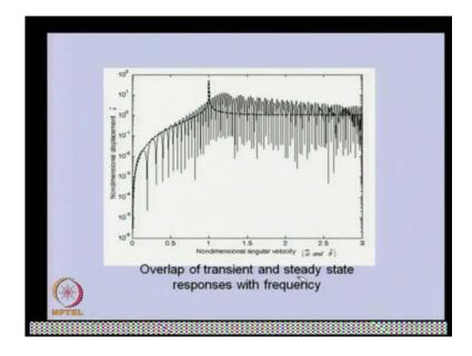
So, you can able to see this is the semi log case. So this is the case, with without transient and with acceleration, angular acceleration we have we overlapped these 2 responses in 1, for compression purpose.
