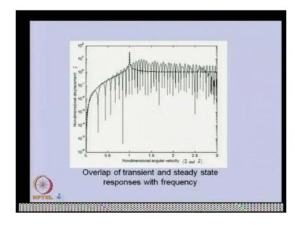
So, this the steady state response, overlapped with the transient response.
