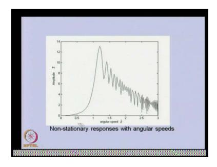
And this is the non stationary response, with angular speed. So, how the amplitude x is changing with x dot x-prime is changing with angular speed.
