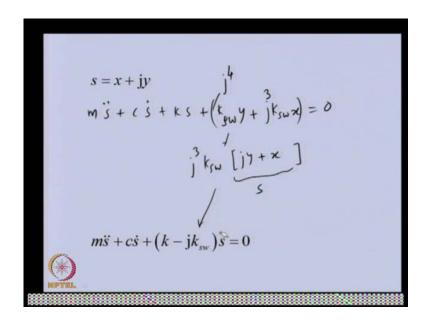
And now, we will we will try to solve this equation, by in the form of complex displacement, which we have to find as x plus j y. So, with this we will multiply the second equation by j and add it to the first equation. So you can able to see that the first term will be simple. ms double dot plus c s dot. So, this is the first 2 terms, will give this. And then, this K x and K this K x and K y, will give this. Then, K s w that is for steam whirl, x plus minus K s w j y is equal to 0.
