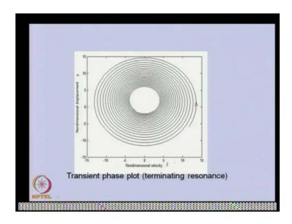
And once we cross the resonance, this is a terminating resonance, so it is coming down. This is the steady state response with time, for particular frequency. So at one particular frequency, if we are not having acceleration, this will be in the form of response.
