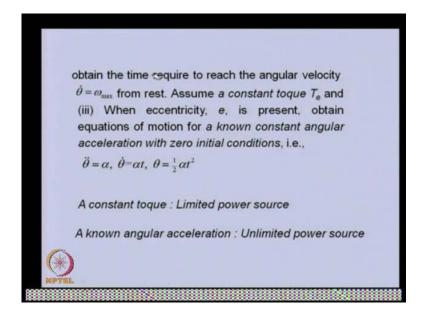
This what will be the basically, time required to reach the angular velocity. Whatever the maximum velocity from rest, how much it time it take to reach that up to that point. In this particular case, we assume the torque as constant and another case when the eccentricity is present in the system, will be obtaining the response, for known constant angular acceleration, with some 0 initial condition.
