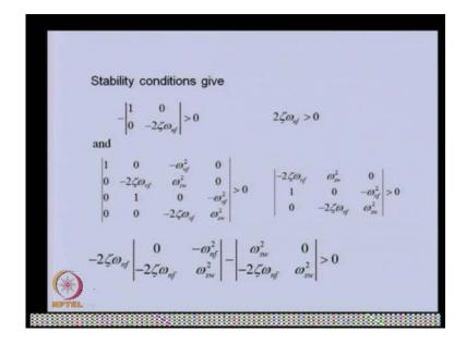
So, from first condition this determinant if we are putting 0, we are getting this condition from second one, after simplification we will get this condition, that k s w by k should less than 2 zeta which is damping ratio.
