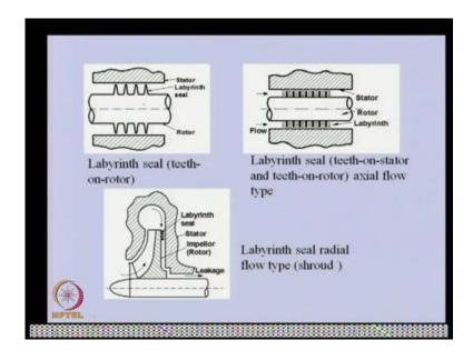
And similarly, we can have the labyrinth seal on the rotor, instead of stator. And basically, they are all over the circumference and we will see, we see that the, this prevent the leakage of the fluid, because of the various abstraction. Sometimes, this labyrinth seals are provided in not only in the stator, but also in the rotor. So that the path of the working fluid or lubricant is zigzag, while it when it is passing through this.
