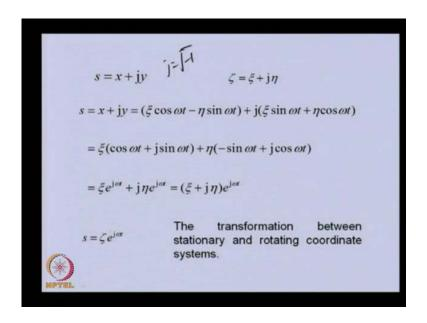
Now, we are defining a complex displacement s which is defined as x plus j y. j is the complex quantity that is root of in the rotating coordinate system. Similarly, we are defining zeta is equal to xi plus j eta s. xi are the complex coordinates in stationary coordinate and rotating coordinate system. Now, this two in place of x and y; from previous expression, we can able to write this in terms of zeta xi and eta. Similarly, y we can able to write in terms of this two.
