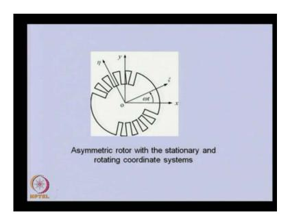
Now, let us see this. If we attach a rotating coordinate system along the two principle direction of the rotor and if we analyze the equation of motion in this rotating coordinate system then it will be convenient to analyze. So here also, we will be choosing the rotating coordinate system. We will be obtaining the equation of motion in the rotating coordinate system itself. In fact, we will be defining the stiffness of the shaft in these two directions in the rotating coordinate system itself.
