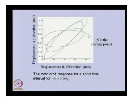
This is the orbit plot that means, x direction and y direction displacement plot with respect to time. So, we have given some initial disturbance. So, this is the initial condition. From here we have leave we are leaving the rotor. So, it is going like this. It is trying to stabilize. So, this is for very short duration of time.
