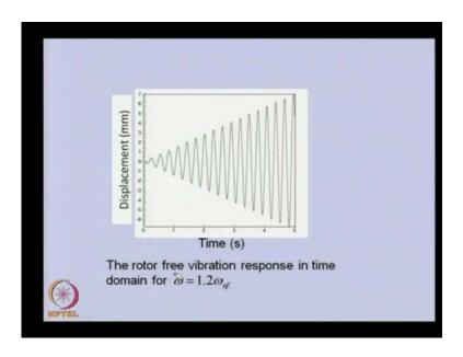
For a given initial disturbance, the amplitude grows with time.
