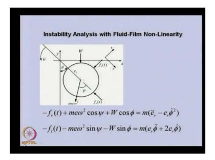
So, here briefly I am outlining how the instability analysis can be done for fluid film force. If non-linearity we want to consider so in this particular case, this is the rotor. In this, we have fluid film forces in two directions; radial direction and the tangential direction. Weight of the journal is here. This could be unbalance force which is rotating with some speed. The position of the rotor is given as eccentricity and the altitude angle.
