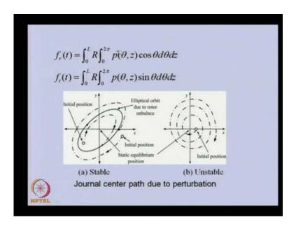
So, over the inside the surface of the bearing from 0 to 2 pi angle and from the length of the bearing, we need to integrate this pressure, which we can obtain. This pressure, we can able to obtain from the Reynold equation, so component of these pressures in the radial direction.
