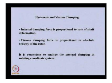
Now, coming to the difference between the hysteretic damping and viscous damping. Internal damping force, which is nothing but hysteretic damping is proportional to the rate of shaft deformation. But, the viscous damping is proportional to the absolute velocity of the rotor. So, one is rate of shaft deformation. Another damping force is proportional to the absolute velocity of the rotor because of this internal damping direction changes along the shaft rotation.
