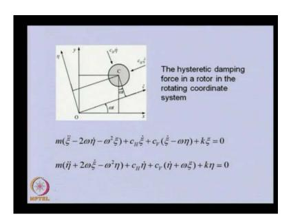
Now, coming to the hysteretic damping; here, this is the xi direction. This is the eta direction. We have earlier noted that the hysteretic damping or internal damping; it acts proportional to the rate of deformation of the shaft. Because this coordinate system xi and eta is attach and is rotating with spin speed, so the rate of deformation of the shaft will be xi dot and eta dot.
