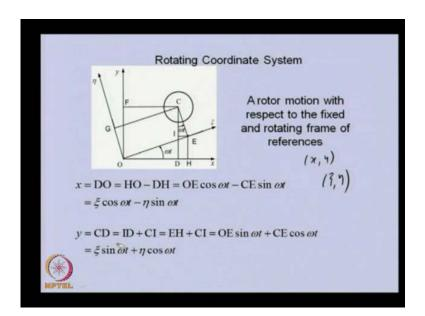
So, x y is stationary coordinate system. Psi and eta is rotating coordinate system. We want to transform the equation of motion in x y, x's coordinate system to the rotating coordinate system. Before that, we can able to relate these two coordinate system. So, with elementary geometry, we can able to relate that. Here, you can able to see. This is
