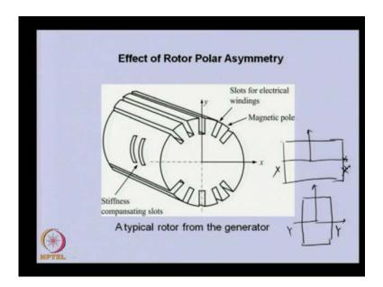
So, this is a one particular a typical rotor of the generator, in which you can see there has slots which are running axially. These are provided generally for providing windings in the generator. Here also it is, but some part of the rotor is solid. So, we can expect that in this particular case, the effective area of the shaft will be something like this because we have removed the material. So, it will be something like this.
