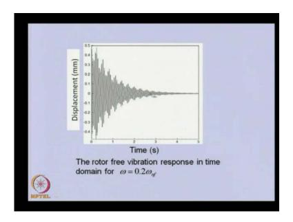
We can use any numerical integration method. This is the displacement with time when we are considering the speed is equal to 0.2 of the natural frequency of the system. Because there is no excitation in the system, so we have given some initial condition, so that once we have disturbed the system, we will see that it stabilizes after some time.
