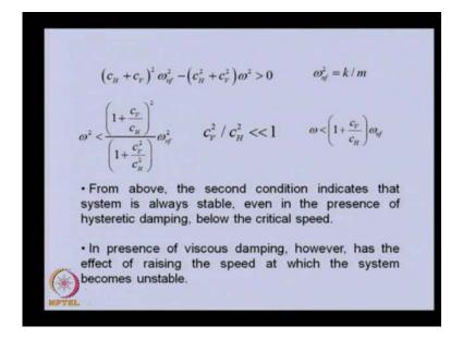
So, if we substitute various coefficients and if we simplify this, we will get expression like this in which we have defined the omega n f square as k by m. In turn, this can be written as omega square less than this quantity. Because this ratio is generally small, so this can be neglected. So, if we neglect this, we will get. Basically, if we take the square root the speed when it is less than this quantity, we will be having system stable. That means when there is no damping in the system.
