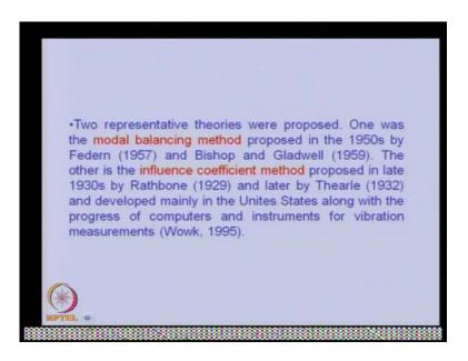
The most important fundamental courses to reduce unstable vibration is liberate geometric imbalance in the rotor. The balancing region of the rotor is relatively early, the particle balancing machine based on this technique was invented in 1907. The arrival of high speed rotating machine made it necessary to develop a balancing technique of flexible rotor.
