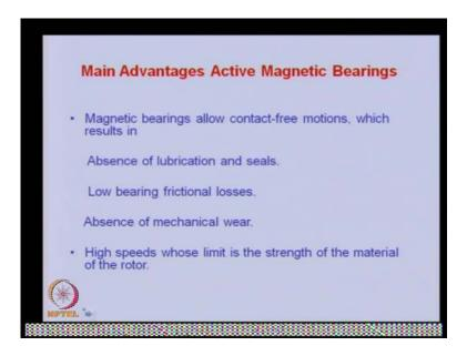
So, this is one of research area which is reactive we know the advantage of this bearing, that because the rotor flows on the air. So, there is no lubrication and friction is less. There is no mechanical and generally only the high speed whose limit is the strength of the material. There is no problem in the, such speed constant by the this particular bearings frictions on the rotors strength should be enough to have that much speed.
