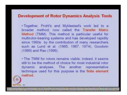
Together, Prohls and Myklestad let to a broader method transfer matrix method of TMM. This method is particular suitable for useful for multi rotor varying systems and has developed rapidly since 1960s by the contribution of many researches including Lund, Goodwin, Rao, etc. The TMM or the transfer matrix method rotor remains viral, indeed it seems still to be method of choice for most hysteria dynamic analysis, the another representative technique for the purpose of finite element method.
