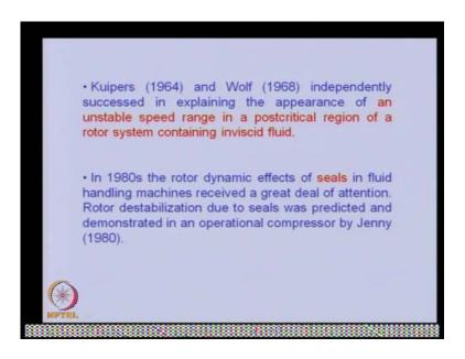
Kuipers in 1964 and Wolf in 1968 independently succeeded in explaining the appearance of an unstable speed range in a post critical region of a rotor system containing in viscid fluid. In 1980 the rotor dynamics effects of seals in fluid handling machine received a great deal of attention. Rotor destabilize due to seal were predicted and demonstrated in an operational compression by Jenny in 1980.
