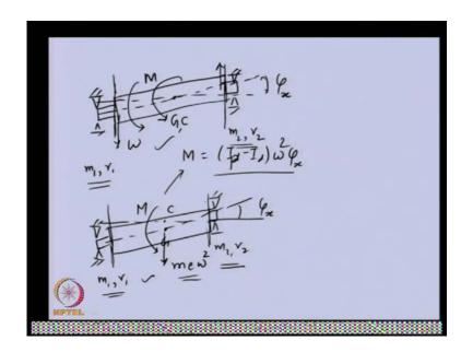
Let us say this the original axis of the bearing and shaft tasks is incline by a shaft term angle producing this angle is. So, the rotor is basically inclined, divide this and execarute the inclination just to show this particular incretion in this the center of gravity is there on the bearing axis.
