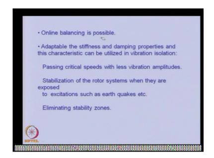
With this magnetic bearing, not only we can suppress the redolence only, also we can able to have a online balancing because we can adaptable the stiffness and damping property online. And this are the some other advantage like we can able to eliminating stability this is some, also in last two lectures we are see introduction to the rotor dynamics. We are seen in the history of rotor dynamics, even in the state of the art in the rotor dynamics brief to these lectures.
