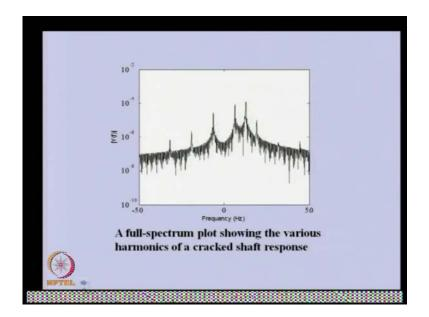
It is a typical full spectrum plot showing the harmonic, even the can able to the frequencies are there, not only in the positive side, also the negative side. We have seen earlier the concept of the forward hold and backward hold. You can able to see the some frequencies components which are negative side belong to the backward hole and positive side to the forward hold.
