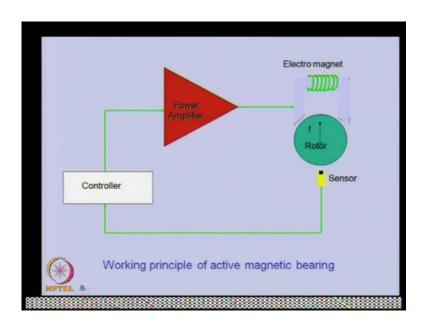
This is a magnetic bearing active magnetic bearing, this is rotor which is floating on air. The sensor measure it is vibration and it gives to the controller. Controller gives the acquired current to the and this amplifier gives the current. This actuator, so that required current can be given to the active vector and this will produce magnetic field to pull the rotor up and down, depending upon its motion. So, this is actually active magnetic bearing.
