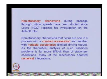
The non-stationary phenomena during passage through critical speed have been studied since Lewis in 1932 reported the investigation on the Jeffcott rotor. Non stationary phenomena that occur are one in a process with the consent and acceleration and another with a variable acceleration. In which we have limited the driving top at the critical analyses with conditional process is the former difficult, than the conditioner exultation many of the researches doctored memorical integrations.
