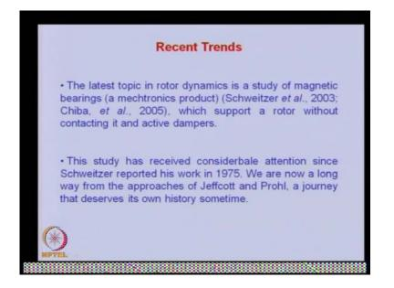
So, the latest topic in the rotor dynamic is the study of the magnetite bearing is a mechtronics product and which supports the rotor without contacting it and active damp fluids damping effect. This study was reviewed considerable attention since the work reported in 1975. We are now long from the approaches of Jeffcott and Prohl, a journey that deserves its own history sometimes.
