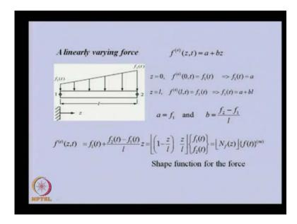
Based on the lump force analysis and other case, let us say if the force is linearly varying like this amplitude of this are given because it is linearly varying. So, let us express the force as it is a linear polynomial where a and b are constant to be found out from the end condition of the force distribution. So, at z is equal to 0 the amplitude of force is f 1, so if we substitute here we will get a is equal to this one for z is equal to L, here the amplitude is f 2.
