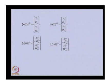
Now, these equations, now let us see the nodal displacement so this is corresponding to element 1 and this is corresponding to element 2 and this is force factor for element one and element 2.
