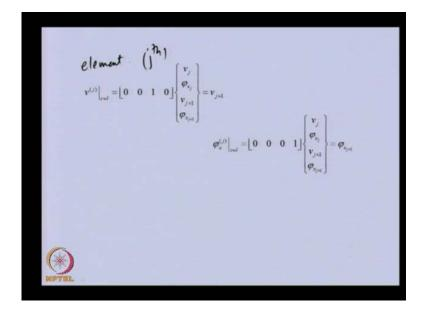
So, for z is equal to L for first element 1 that is a z is equal to L, so we are getting if you substitute in the previous expression this expression z equal to L we will get only this as 1 other are 0. So, we will get v is z plus 1 and slope we will get phi x z plus 1, so this is for element in this particular case j th element this is j th element, now for j plus 1 element, this is the expression, so this was a z plus 1 element.
