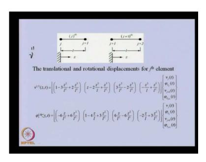
These shape functions are giving same translational displacement as well as slope that mean there comparability up to that. If you want to check for higher order, then will see that this may not be this shape functions may not be comparability for second derivative. So, if we take derivative of this once more and predict the value at common nodes from this two different elements will see that they will not match. (Refer Slide Time: 28:54)
