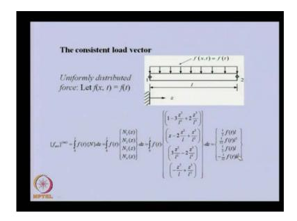
So, in the first case let us say we if you want to obtain the consistent node vector for uniformly distributed load that is so f t is a load, which is uniformly distributed over the element. So, this is the load per unit length. So if we if we substitute this in the distributed load component they is no concentrated force because that was containing 2 terms one was distributed and another was concentrated, so this only we considering the distributed one.
