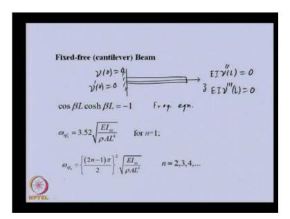
Now, let us see some other boundary condition, how the frequency, the natural frequency and Eigen function take the shape? So, this is a fixed free beam, that is cantilever beam. In this particular case, we have boundary condition that this is a fixed end, so we will be
