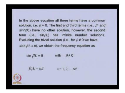
So, this is the solution. So, this is the infinite number of solutions which is possible for which sin beta value is 0. So, if you substitute this for all, we can be able to get these values. This is equal to 0 value.
