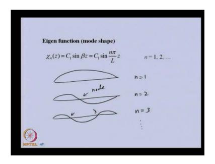
So, this will give us the Eigen function. So, out of 4 terms only single term is left out. This is the C 1 and beta which we have already obtained in terms previously. So, that we can be able to substitute here. So, this is the Eigen function, where n can be 1, 2, 3 and 4. This Eigen function is nothing but the mode shape. We can be able to draw the mode shape. How the beam will vibrate in simply supported case? Let us say for mode 1, that is n is equal to 1.
