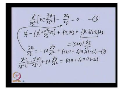
So, this is one of the equation. This we obtained by moment balance. Now, we can be able to do the force balance. For force balance, we have sheer force, external force and inertia force. So, these we can be able to create keeping the sign. So, force balance S y is in positive direction and the change in that is in negative direction. So, this and then we have external force which is distributed. If you have concentrated force, that also we can be able to incorporate in this.
