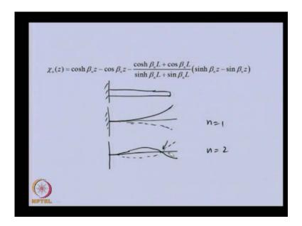
So, this is the Eigen function. If we plot this, we know that the mode shape for this particular case. Let us say for n is equal to 1, if this is the centre line we will be having mass, because at this end we have slope and linear displacement 0. So, while drawing the
