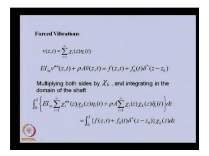
So, now we are trying to solve the forced vibration. So, this is the governing equation which we derived earlier in which, now we are considering the force. This is a distributed force and this is the concentrated force. Summation of this now, we are
