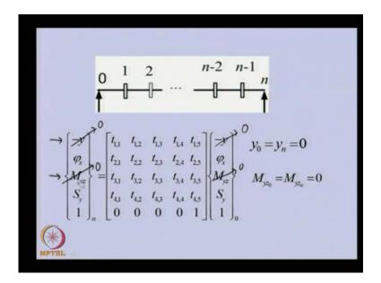
So, like this, so this is the nth station zero station. In the previous overall transverse matrix t relates the state factor here to the state factor here. Now, that particular last equation expanded here. So, this is state factor at nth station, these is the state factor of 0 station and because if there is unbalance in the system, the form of the overall transfer
