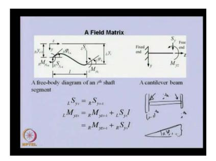
Now, in the second case will consider the shaft as recite and then will give the these two displacement. Now, this y and pi displacement to the this end of the shaft which is now in the second case we are considering as recite. We can able to see that whatever the displacement of the ith minus 1 right of i minus because disc is there linear displacement, same will be there. Put this value here and for the slope for slope again we need to refer the figure for slope.
