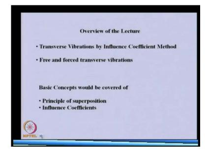
Now, let us see, what are the things we will be covering? So, apart from the methods, which we covered in the previous cases for torsional vibration one important method, the influence coefficient method which will be covering for transverse vibration and both free and force vibration can be analyzed using this particular method. Basic concepts, which we will be requiring for this is principle of superposition, basically will be dealing with the linear system.
