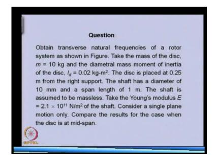
Now, various property of this are given here mass is 10 k g i d is 0.02 k g meta square disk location is also given that from right support it is 0.25 meter and total length of the
