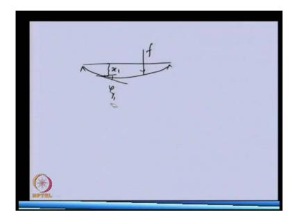
We know that if we are applying a force in a simply supported beam, if we applying some force not only it gives the linear displacement. Let us say at this location this is in the x 1, but also it gives the slope because original heat slope was 0. But now the slope has changed some angle. So, the force normally gives the linear displacement, but also the angular displacement simultaneously.
