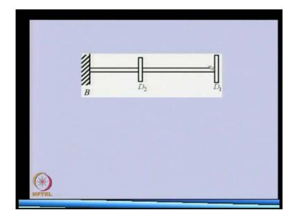
So, we have a rotor system like this in which we have two disks, mass of the shaft we are not considering. We are considering that the disk is having mainly the up and down tilting motion linear motion. Tilting motion we are ignoring it.
