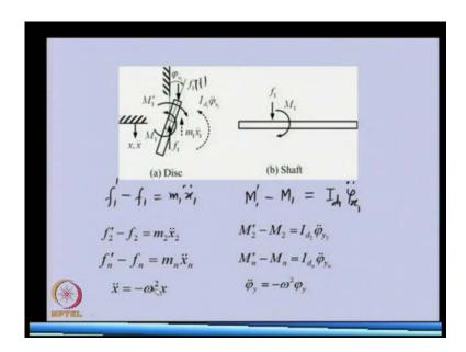
So, this is basically a free body diagram of a disk when this several forces or movements are acting, but let me first introduce the alpha 1 sorry f 1 prime f 1 prime. This is the external force, which is acting on the disk this is the external force, this is time dependent. So, basically now all the forces are time dependent. Similarly, we have movement which is external movement time dependent. This may come if disk is not perfectly perpendicular to the shaft, if it is slightly tilted.
