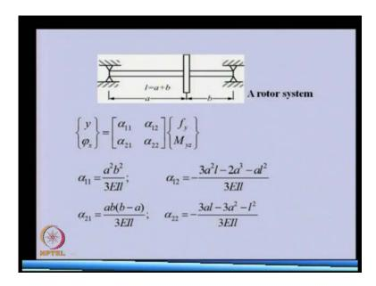
Very simple rotor like this we have we have considered this is simply supported rotor system mass of the shaft. We are not considering only the inertia of the shaft is there and we are considering both mass and diameteral mass movement of inertia of the disk. (Refer Slide Time: 28:25)
