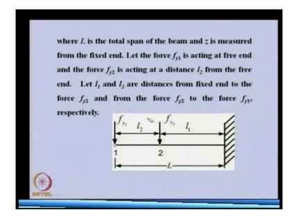
So let us see, how it can be done? So, two forces are acting, the first force distance from the fixed end is 1 1. This is between two forces, the distance is let us say 1 2 total length is 1.
