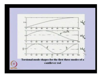
So, this is the plot of the Eigen function. So, you can able to see this is the position of the shaft this is the fixed end of the shaft and this is the free end of shaft and this is the angular displacement and this is a relative angular displacement. So, we have taken the
