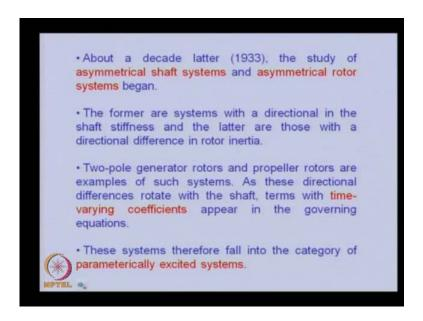
So, after the Jeffcott's analysis about a decade later in 1933, the study of shaft system and asymmetrical rotor system began. This two rotor systems, we will see what are the differences between them? The former are systems with a directional in the shaft stiffness. The symmetrical shaft system is in which there is the directional in shaft stiffness. That is the shaft stiffness changes with the direction as it rotates.
