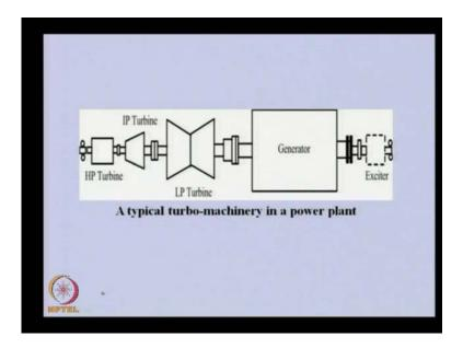
If we have multi staged turbine, then we can have high that is high pressure turbine, low pressure turbine and generator and all are connected by coupling and supported at various bearings here. Even you can be able to see the exciter. So, these all are nothing but rotors, which are mounted on bearings.
