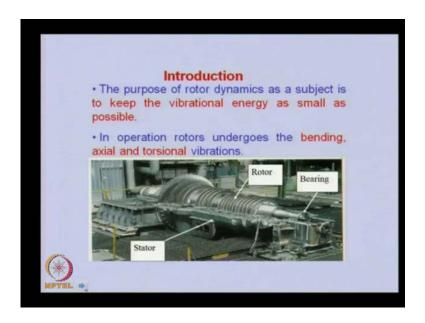
Now, let us see endow steel rotor that is also having similar components, but they are having huge size. You are able to see the bearing here and rotors and various stages of the blades stator foundation which will be mounted on a heavy concrete structure. So, you can able to see that the main purpose of the rotor dynamics as rotor dynamics as a subject is to keep the vibrational energy as small as possible. In operation, rotor undergoes the bending, axial and torsional vibrations.
