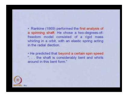
Rankine in 1869 performed the first analysis of a spinning shaft. He chose a two degrees of freedom model consisted of a rigid mass whirling in an orbit, with elastic spring
