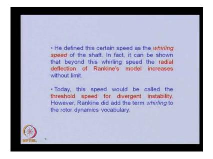
He defined this certain speed as the whirling speed of the shaft. In fact, it can be shown that beyond this whirling speed, the radial deflection of rankine's model increases without limit. So, it goes to an unstable region. Today, this speed would be called the threshold speed for divergent instability. However, rankine did add the term whirling to the rotor dynamics vocabulary. So, whirling was first was used by rankine. His analysis was having some flop as we will see in subsequent style.
