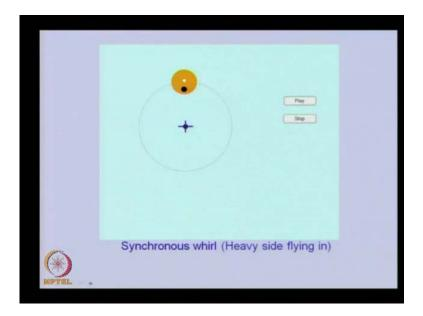
This is the animation in that in which the rotor is whirling. Generally, this will occur when we are operating about the critical speed, heavy side will be inside all the time and because of that, you can see that vibrations will be less because the unbalanced force will be towards the bearing access.
