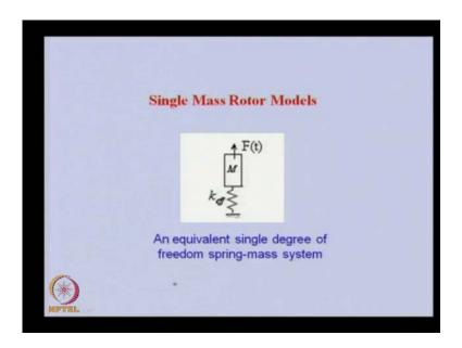
Basically there is nothing but a single degree of freedom mass system in which that particular model can be analyzed. It is the very basic model of spring and mass temper, system temper is not there in this an external whirling due to the unbalance.
