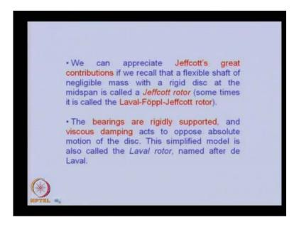
We can appreciate Jeffcott's great contributions if we recall that a flexible shaft of negligible mass with a rigid disc at the mid span is called a Jeffcott rotor in rotors dynamics community. Sometimes it is also called the Laval Foppl Jeffcott rotor. The bearings are rigidly supported, and viscous damping acts to oppose absolute motion of the disc. This simplified model is also called the Laval rotor, named after de Laval.
