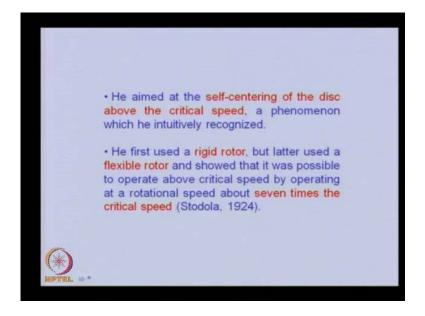
He aimed at the self centering of the disc above the critical speed, which he intuitively recognized that was actually contradicting the Rankine's prediction that you cannot be able to operate this rotor beyond a certain speed, but he was getting in actual centering, self centering of the rotor when it is operating at a critical speed that is it was operating
