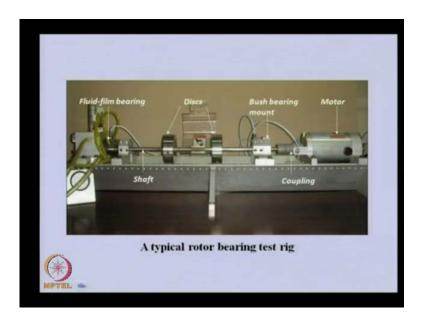
With this figure, I just want to introduce a basic component of a rotor, especially in the laboratory. So, here is a motor, which drives a shaft through a coupling or the shaft is
