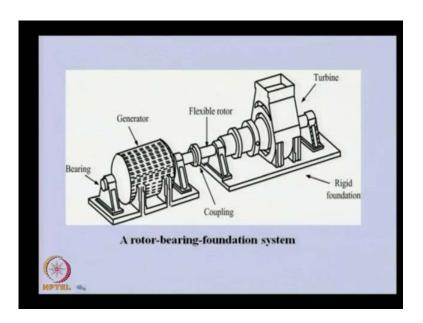
This is very schematic of the same and that is turbine generators at with a coupling in between.
