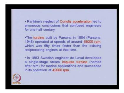
Similarly, in 1883, Swedish engineer de Laval developed his single stage stream turbine that is impulse turbine that is named after him for marine applications and succeeded in its operation at 42000 rpm, which was very high speed at that time.
