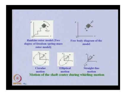
So, this is the subsequent model in which he considered a rotor as the mass and rotor by a spring. Spring has directional change in the thickness. You can able to see that of this particular rotor will be having some orbit. Depending upon the stiffness of this spring, it can have a circular motion or elliptical motion. If there is a cross coupled term and a symmetry in the support, you can have elliptical or in extreme case, it can or elliptical, it can have a straight line motion.
