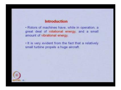
Rotors of machines have, while in operation, a great deal of rotational energy, and a small amount of vibrational energy, which is actually unwanted form. The main aim should be to have as much as have rotational energy minimum vibrational energy. You can able to see that it is very evident from the fact that a relatively small turbine propels a huge aircraft.
