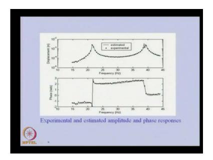
So, this is the typical plot for rotor. You can able to see that this is the spinning speed of the shaft. It is increasing from some from 15 to let us say 45 hertz. This is the displacement. So, whenever the spin speeds was close to critical speeds, there was high amplitude. You can able to see the second plot is a phase plot there is a change in the phase of around pi radians and even at the second critical speed, there was a change in the phase.
