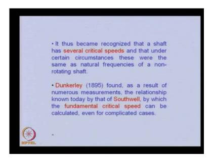
It thus became recognized that a shaft has several critical speeds and that under certain circumstances; these were the same as natural frequencies of a non rotating shaft. Dunkerly in 1895 found, as a result of numerous measurements, the relationship known today by that of Southwell, by which the fundamental critical speed can be calculated, even for complicated cases.
