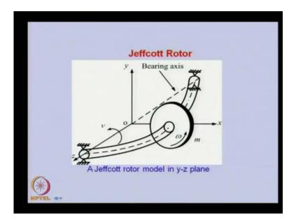
This is a diagram of Jeffcott rotor in which there is a flexible rotor, which is a mass less rigid disc and the bearings are rigid. They allow only the rotational motion of the shaft
