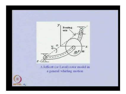
To have more understanding of this, let us see this figure in which the bearing axis and there is the shaft, which is bent. Now, this has bent because of its bending on its own axis
