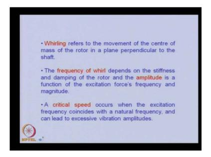
So, now let us see our whirling. It refers to the movement of the centre of mass of the rotor in a plane perpendicular to the shaft.
