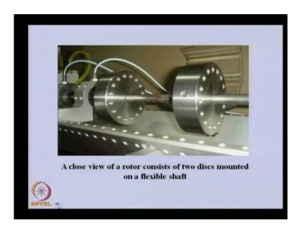
So, here is the close view of the disc. Generally, we provide some kinds of holes in it so that we can be able to provide some kind of unbalanced known and unbalanced to study the unbalanced vibration of the system.
