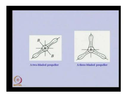
So, we can able to see as this propeller rotates about the fixed axis, their diameter mass movement would change and because of that, there will be the rotor mass asymmetry.
