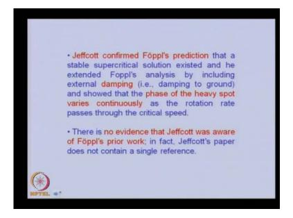
Jeffcott confirmed Foppl's prediction that a stable supercritical solution existed and he extended Foppl's analysis by including external damping that is damping to the ground and showed that phase of heavy spot varies continuously as the rotation rate passes
