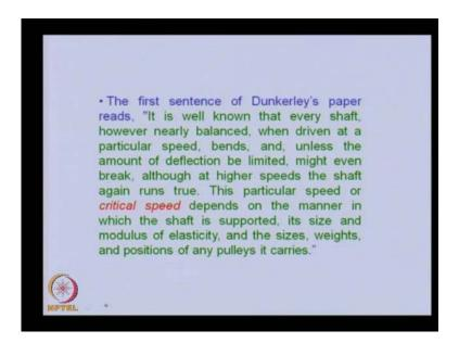
So, this is the first sentence of the Dunkerley's paper, which reads as it is well known that every shaft, however nearly balanced, when driven at a particular speed blends, and unless the amount of deflection be limited, might even break, although at higher speeds the shaft again runs true. This particular speed or critical speed depends on the manner in which the shaft is supported, the size and the modulus of elasticity and the sizes, weights, and positions of any pulleys it carries.
