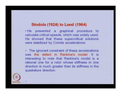
He presented a graphical procedure to calculate critical speeds, which was widely used. In industry, he showed that these supercritical speeds solutions where stabilized by Coriolis accelerations. The ignorant constraint of these accelerations was the defect in Rankine's model. It is interesting to note that Rankine's model is a rational one for a rotor whose stiffness in one direction is much greater than its stiffness in the quadrature direction.
