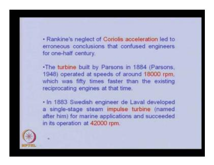
In this particular Rankine's model, as I pointed out, there were some flops in model. So, rankine's neglect of coriolis acceleration led to erroneous conclusions that confused engineers for half, one half century. The turbine built by parsons in 1884 operated at speeds of around 18000 rpm, which was fifty times faster than the existing reciprocating engines at that time.
