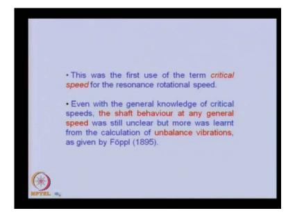
This was for the first time use of the term critical speed for the resonance rotational speed was used. Even with the general knowledge of critical speeds, the shaft was still unclear, but more was learnt from the calculation of unbalance vibrations, as given by Foppl in 1895.
