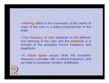
The frequency of whirl depends on the stiffness and damping of the reactor and the amplitude is a function of the excitation force's frequency and magnitude. There is the concept of critical speed also in the rotor. The critical speed occurs when the excitation frequency which comes because of the unbalance coincides with the natural frequency, and can lead to excessive vibration amplitudes.
