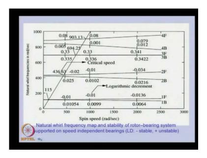
Sometime the Campbell diagram along with the frequency meets at the logarithmic decrements. The size of the logarithmic decrement determines whether the stable or unstable. So, generally whenever it is indicating, the system is stable. If they are positive, the system is unstable. So, with this, we can able to see various modes, so like this, first mode, second mode, which is unstable, after what speed they are unstable, we can able to study.
