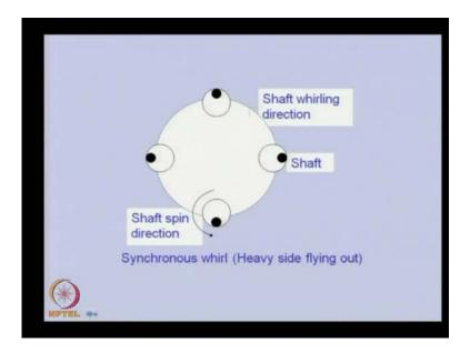
Here we can be able to see that this is the shaft which is whirling; this is the bearing center and the heavy side that means where the unbalance is there is outside. We are considering the synchronous whirl because of that when it rotates along the orbit, always the heavy side will be outside. You can see that the spin direction is counter clock wise and also the whirling also is counter clockwise in this particular case.
