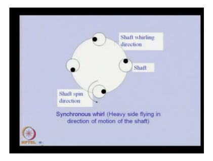
This is another kind of motion in which...actually this is the critical speed. At critical speed, this highly side will be in the direction of motion. So, it will be tangent to the orbit
