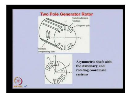
So, let us see with diagram what is two pole rotor. We can able to see this rotor in this generator. Here some slots are there for winding and these are the holes for because of this shaft, the stiffness in one of the plane will be less as compared to another one. To compensate that, some slots are made in other direction also, but still, when such rotor rotates, we can expect there will be change in stiffness with respect to time and that gives parametric excitation to the system.
