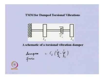
This is a picture of external damper, which is added between two discs and the shaft. Generally here, we this is the damping coefficient. This coefficient multiplied with relative velocity between with this particular shaft will give s the damping force. So, C s and the relative angular displacement at two ends of the velocities, not representing the velocity. So, this will be the damping force of this particular kind of external damper; is a damping force.
