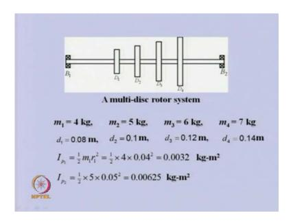
You can able to see. We have four discs. They are connected by uniform shaft. Shaft is supported at ends, frictions is bearing and various properties of this shaft.
