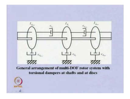
Now, let us see a multi disc rotor system in which number of discs are there and disc because of the working fluid. It is having some kind of damping so that, every place we have added a damper. Damping coefficient of this disc, we are writing as C d, C subscript d. These are for various discs. n minus 1 disc n th disc n plus 1 disc. So, each discs are having some dampers. Apart from that, we have damping in the shaft either in the form of material damping or external damper.
