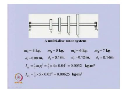
So, you can able to see. There are four discs in different masses. These are thin disc. They have different diameters. So, we are calculated their polar moment of inertial. These are the polar moment of inertial U H.
