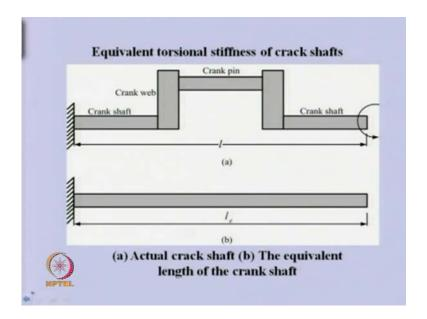
Once we have done it, we can able to convert the reciprocating mass and the revolving mass is purely revolving mass system. Now, let us see the torsional stiffness. Because the crank is having variable geometry so, if we want the uniform shaft so obviously, a equivalent shaft. So, torsional vibration of this system. This system should be same so, we can able to see rather we can do experimentally. We can able to give some twist.
