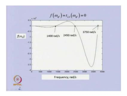
So, for that case, we have once the overall transfer matrix. So, second row and a first column component will give this as a frequency equation. If you expose that as a
