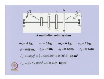
If giving the stations number, station number 1, 2, 3, 4, the state vector which is here right of fourth disc and state vector here right of one disc; they can be related like this.
