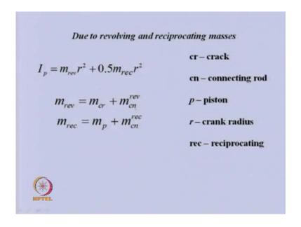
Now, you could able to get what is the equivalent polar moment of inertial of the whole crank connecting rod and the piston.
